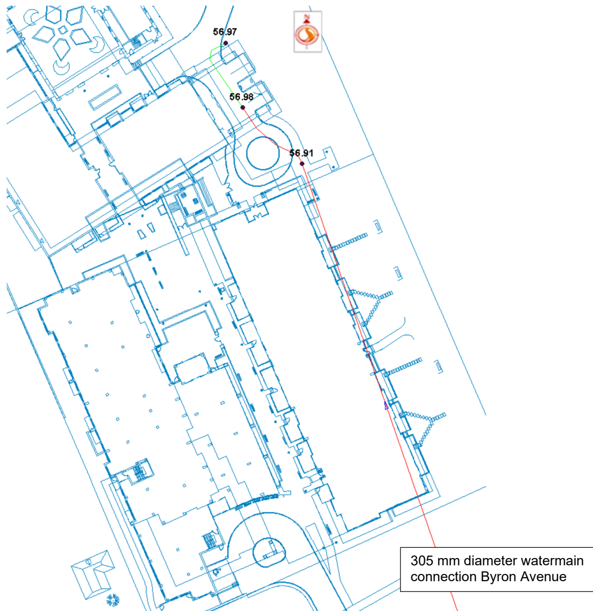
Figure 3-3: Pressures (psi) under PKHR Demands
