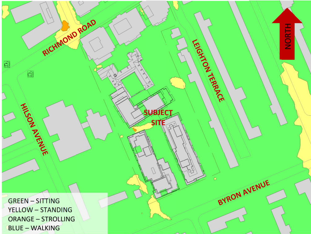
FIGURE 3A: SPRING – WIND CONDITIONS AT GRADE LEVEL
