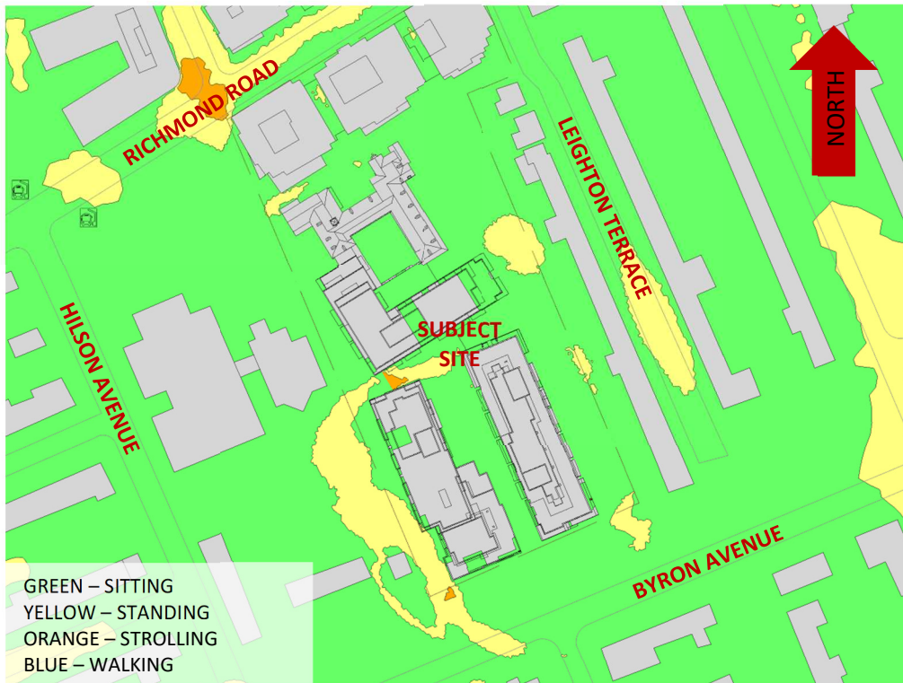
FIGURE 3D: WINTER – WIND CONDITIONS AT GRADE LEVEL
