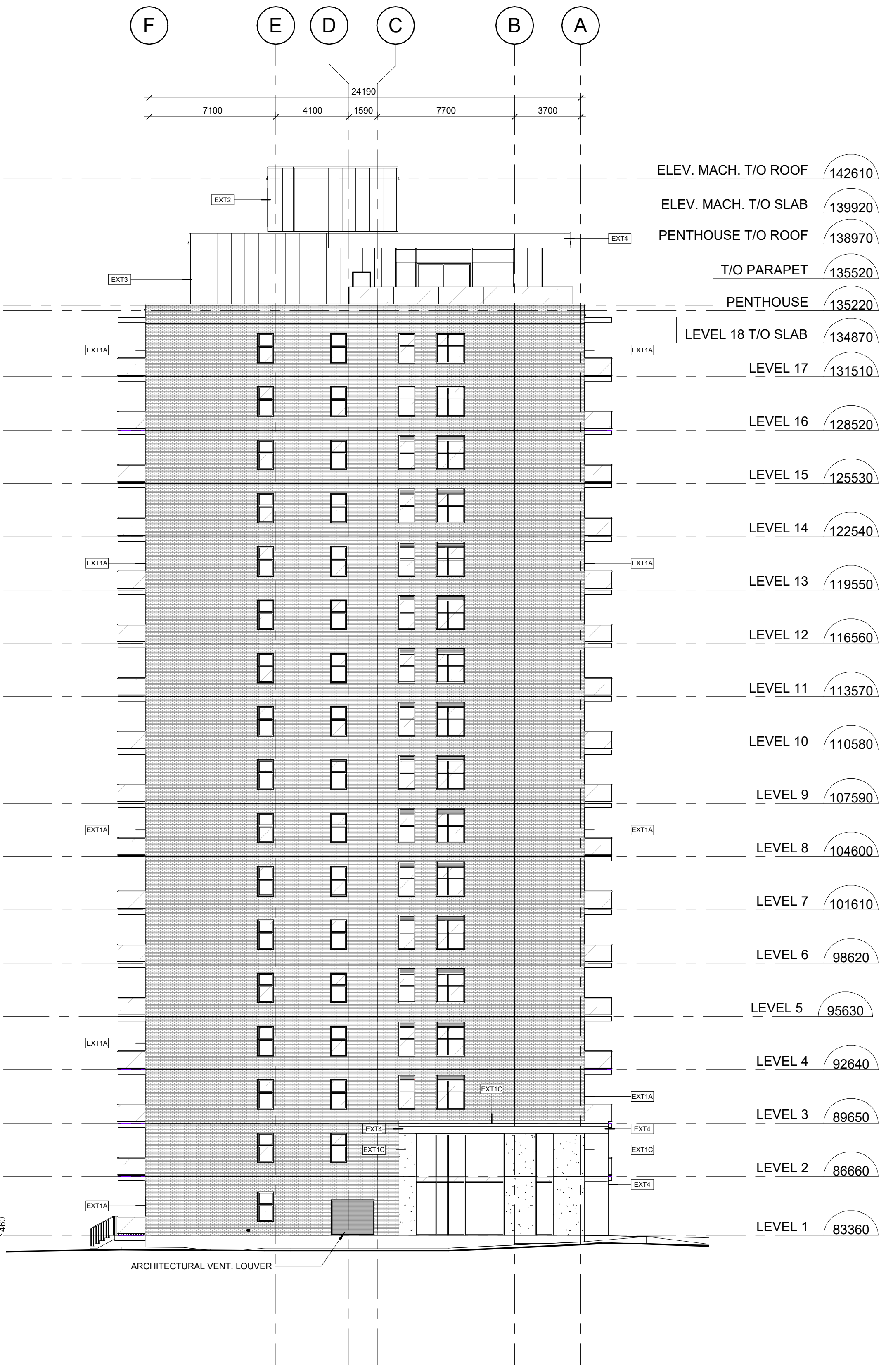
1 BUILDING ELEVATION - WEST SCALE: 1 : 175
