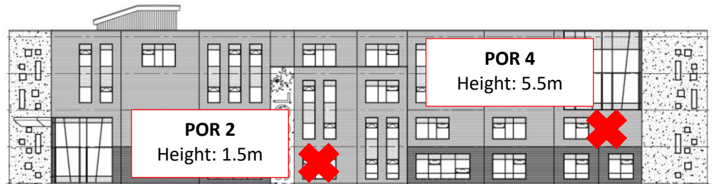
Figure 3.3 – East elevation of Stittsville High School showing location and heights of points of reception.
