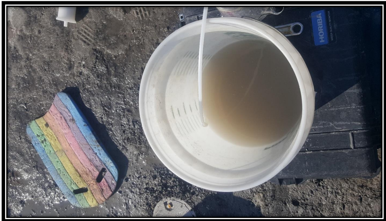
Photograph 6: View of typical purged water during monitoring well development (Feb 18, 2017)
