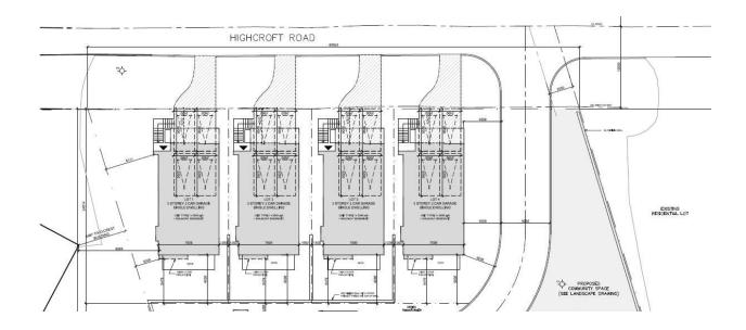
Of importance is that last unit before the existing residential is now 9.956 metres or 32.6 ft between residential units and the distance from the property and the front corner of the new residential unit is now 6.111 metres or 20 ft. which indicates a clear transition from new development and existing.
