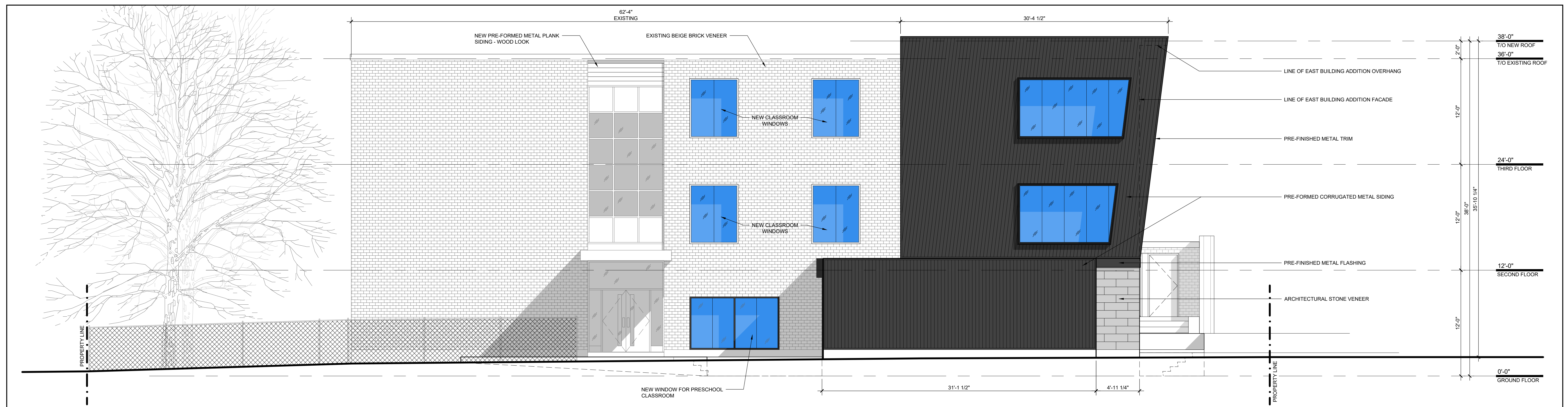
03 PROPOSED BUILDING ADDITION - SOUTH ELEVATION A200 SCALE: 3/16" = 1'-0"
