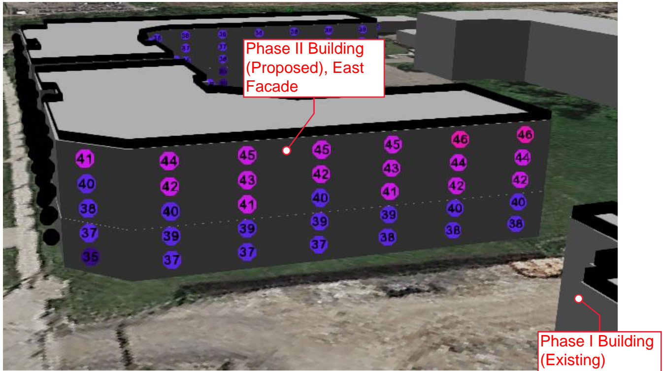
Figure 5d: Impact of Existing Stationary Noise Sources on Proposed Phase II East Façade Facing Phase I, Daytime/Evening Sound Levels, Leq [dBA], Unmitigated
