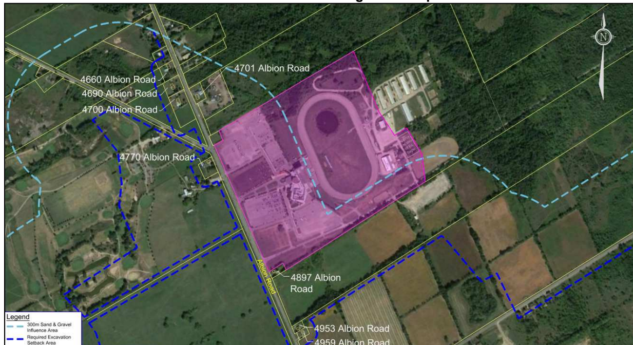
Figure 9. Required Excavation Setback Areas
