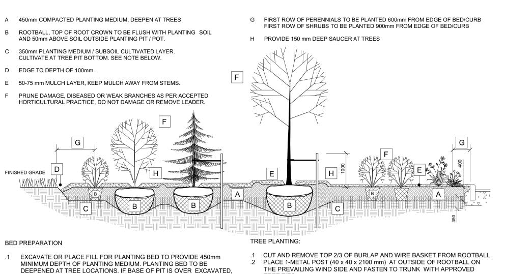
RAISE BOTTOM TO PROPER LEVEL WITH COMPACTED PLANTING MEDIUM. PLACE 150mm PLANTING MEDIUM ON SUBGRADE AND CULTIVATE INTO TOP 200mm OF SUBSOIL. SEE NOTE BELOW. PLACE REMAINDER OF PLANTING MEDIUM OVER CULTIVATED PORTION
