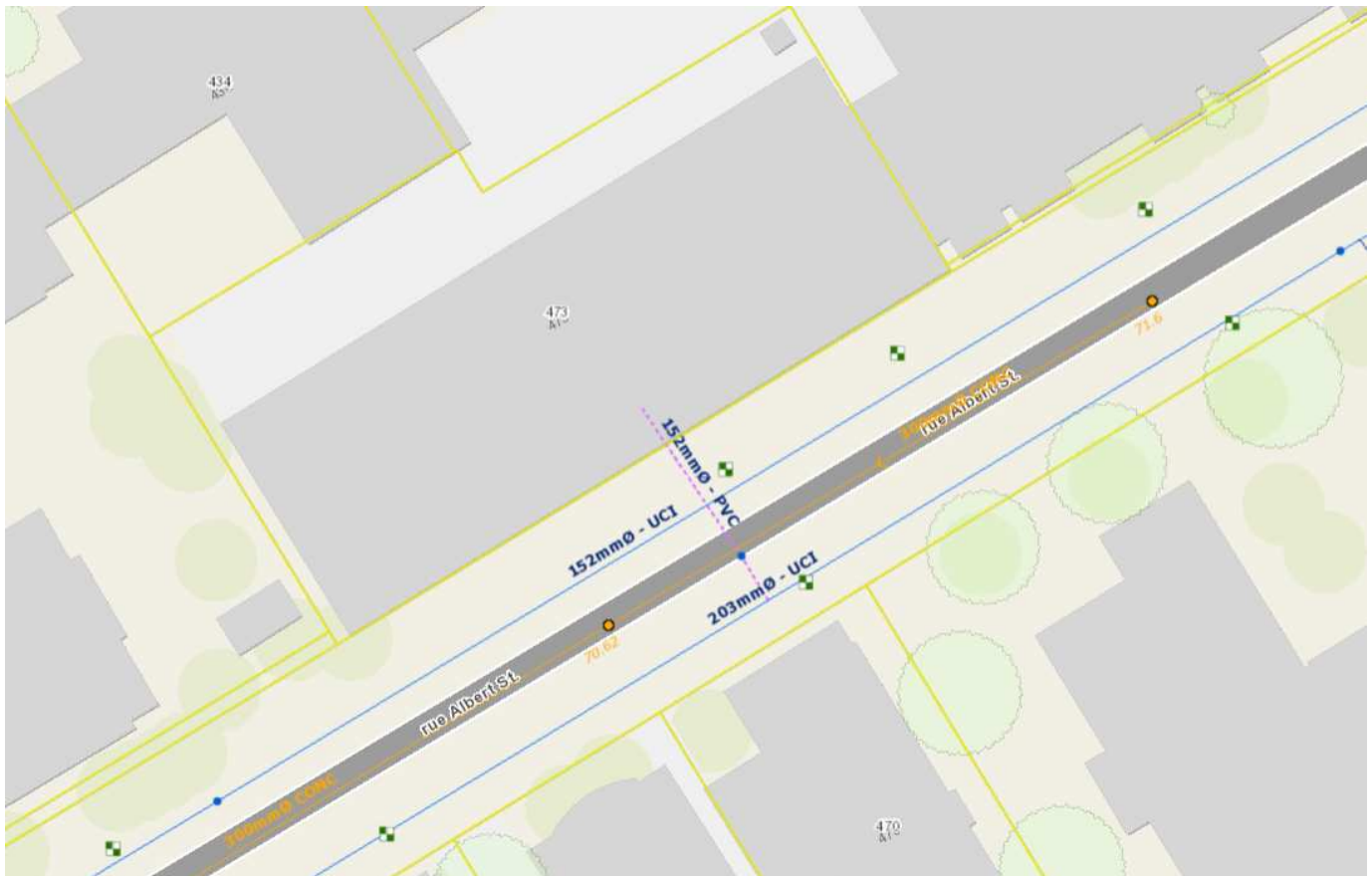
Figure 2: Existing Municipal Infrastructure Surrounding the Site
