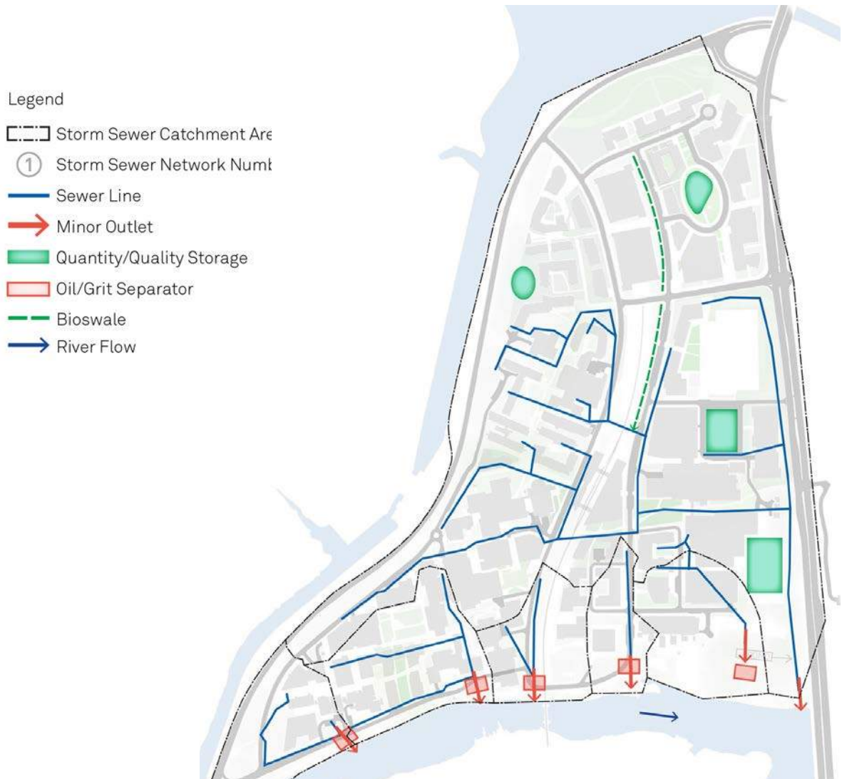
Diagram showing storm sewer and quality/quantity control
