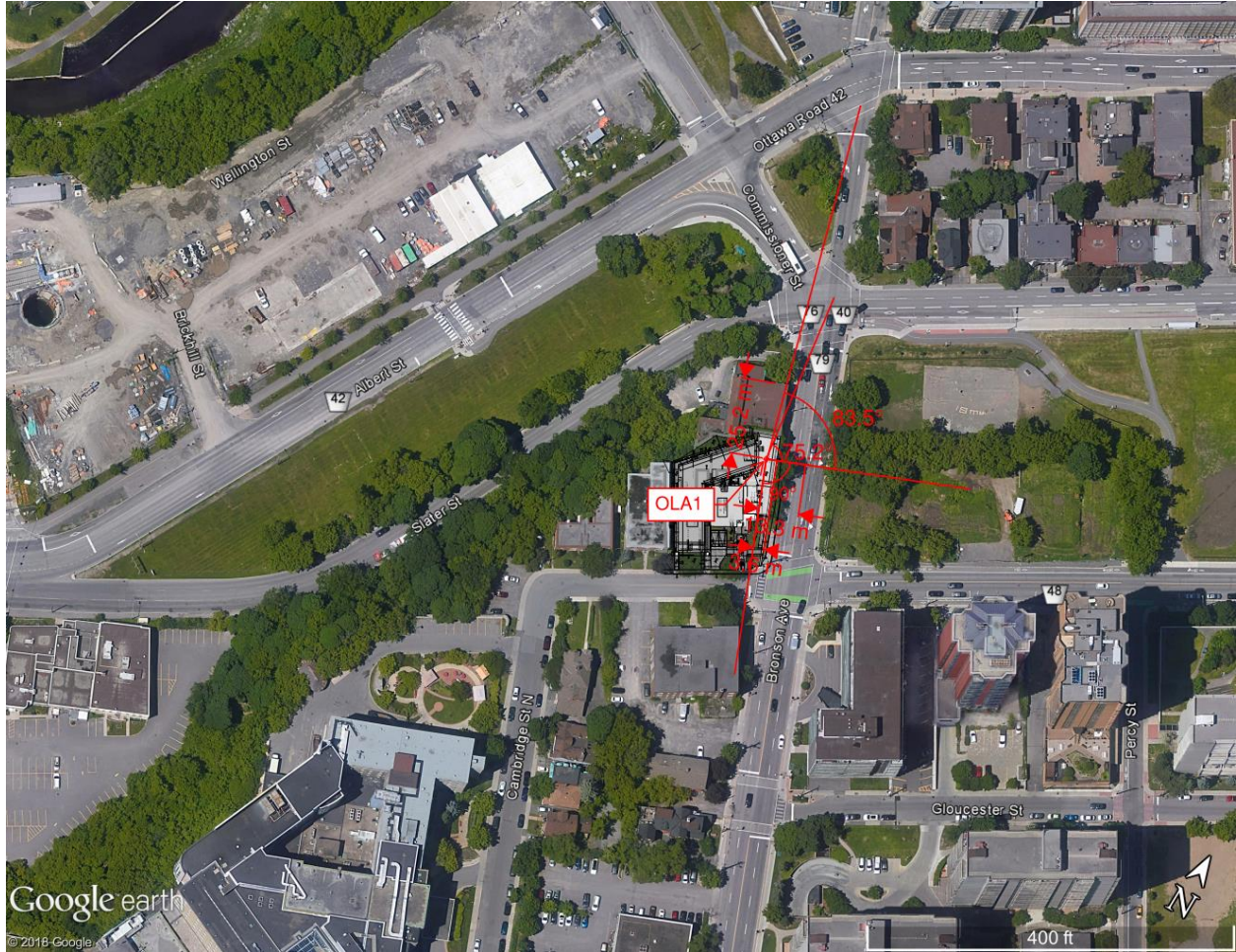
Figure 23: Distances and angles used in STAMSON 5.04 for OLA1 (2 of 3)
