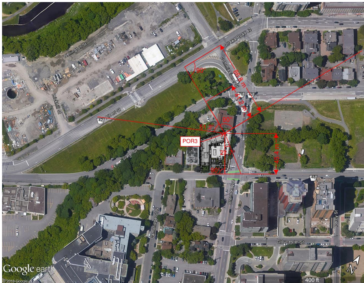
Figure 12: Distances and angles used in STAMSON 5.04 for POR3 (1 of 3)
