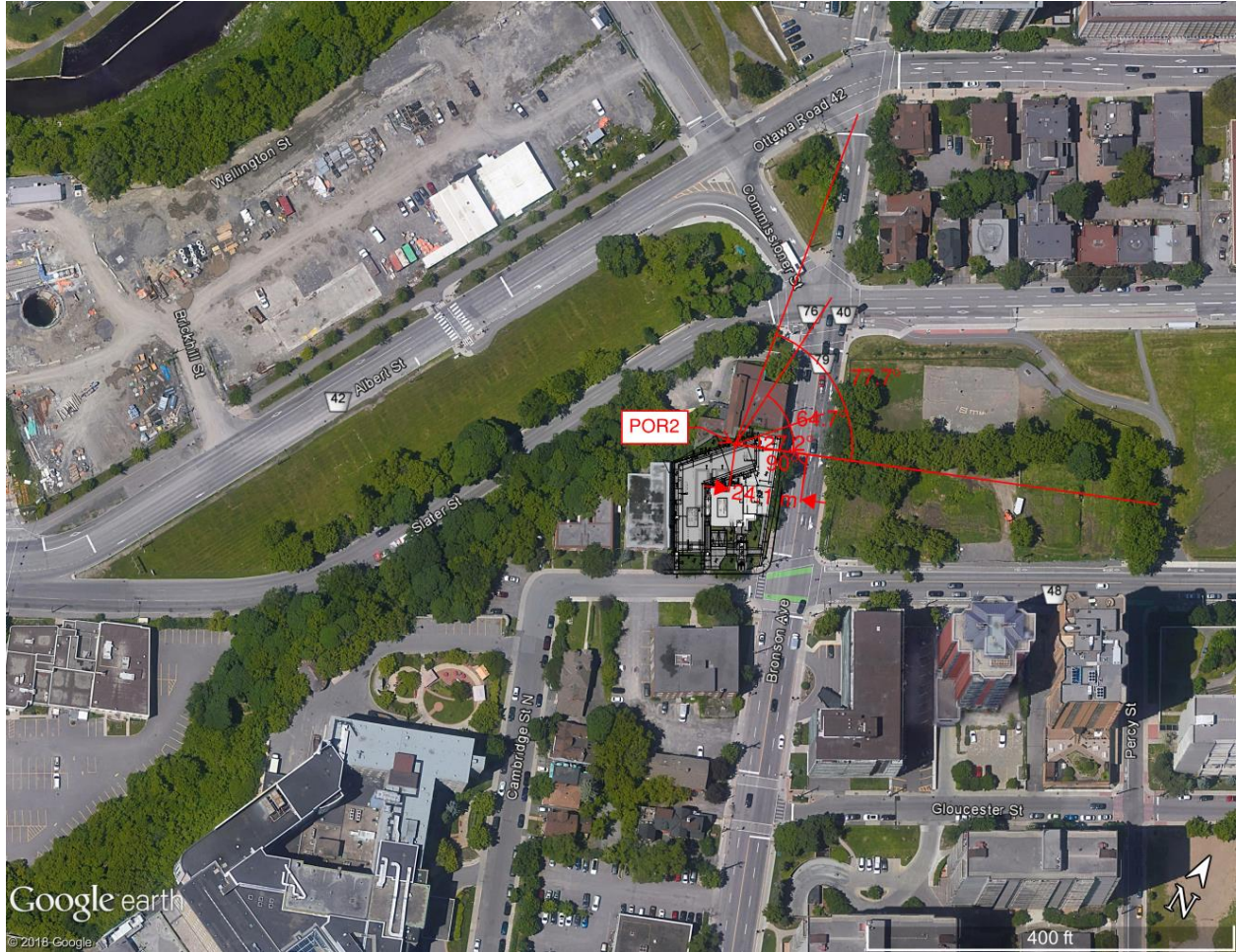
Figure 10: Distances and angles used in STAMSON 5.04 for POR2 (2 of 3)
