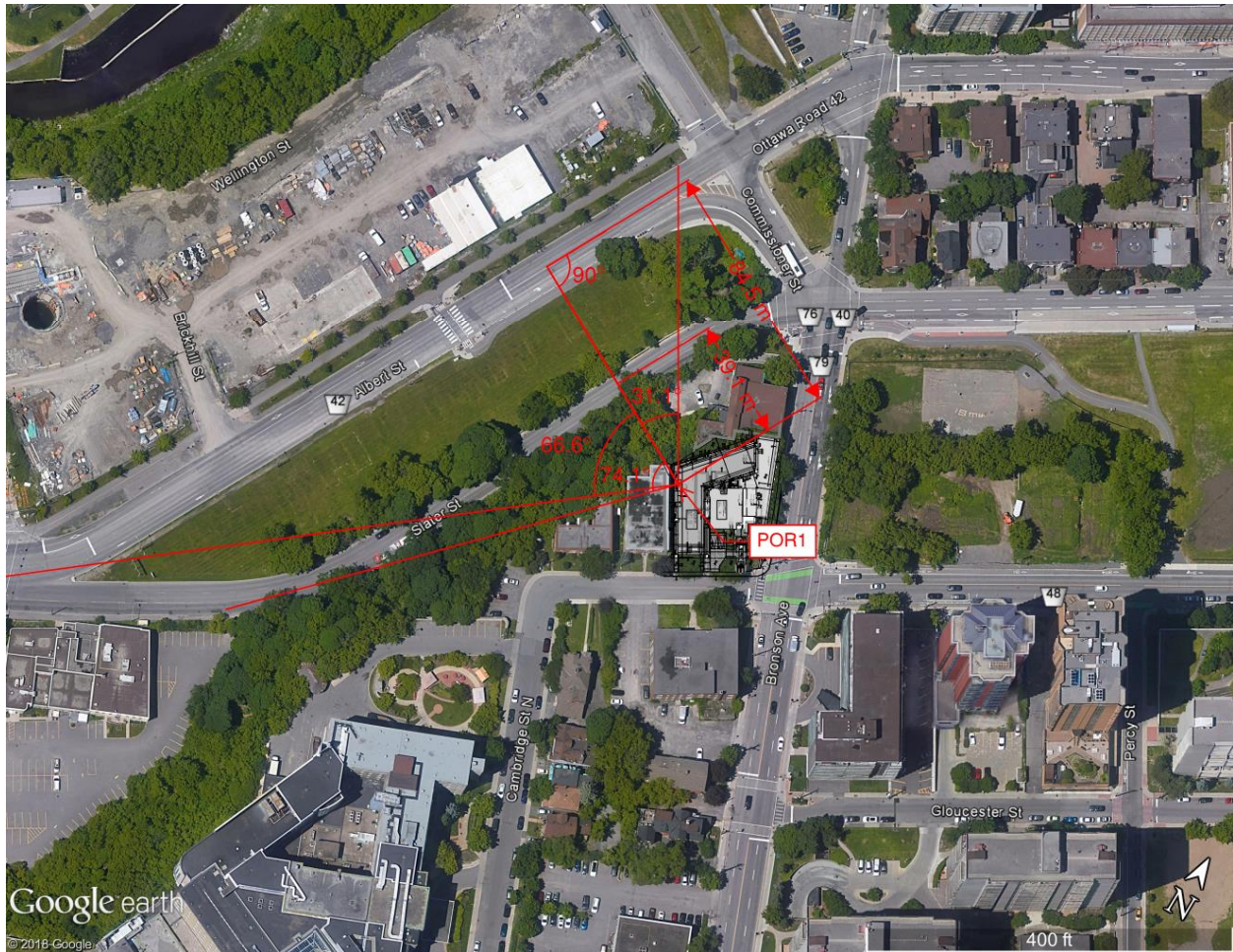
Figure 8: Distances and angles used in STAMSON 5.04 for POR1 (1 of 1)
