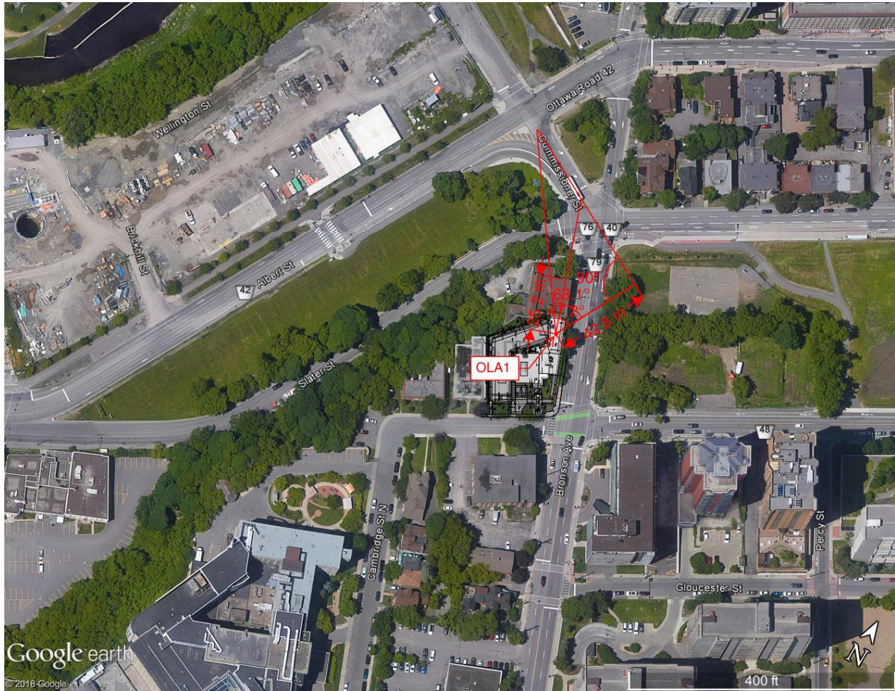
Figure 24: Distances and angles used in STAMSON 5.04 for OLA1 (3 of 3)
