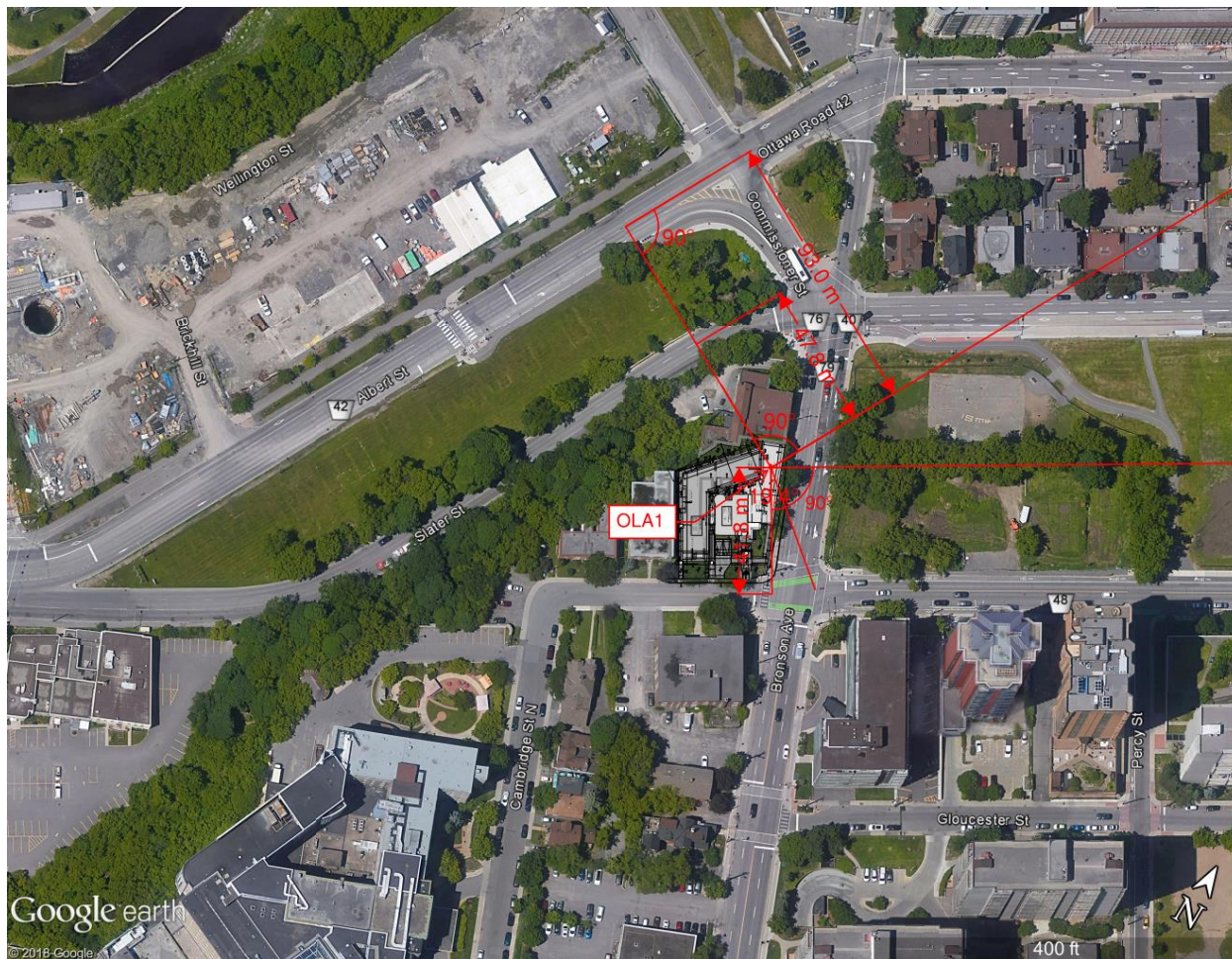
Figure 22: Distances and angles used in STAMSON 5.04 for OLA1 (1 of 3)
