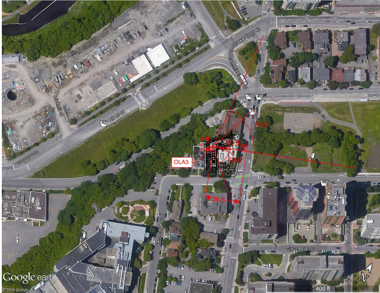
Figure 29: Distances and angles used in STAMSON 5.04 for OLA3 (2 of 3)
