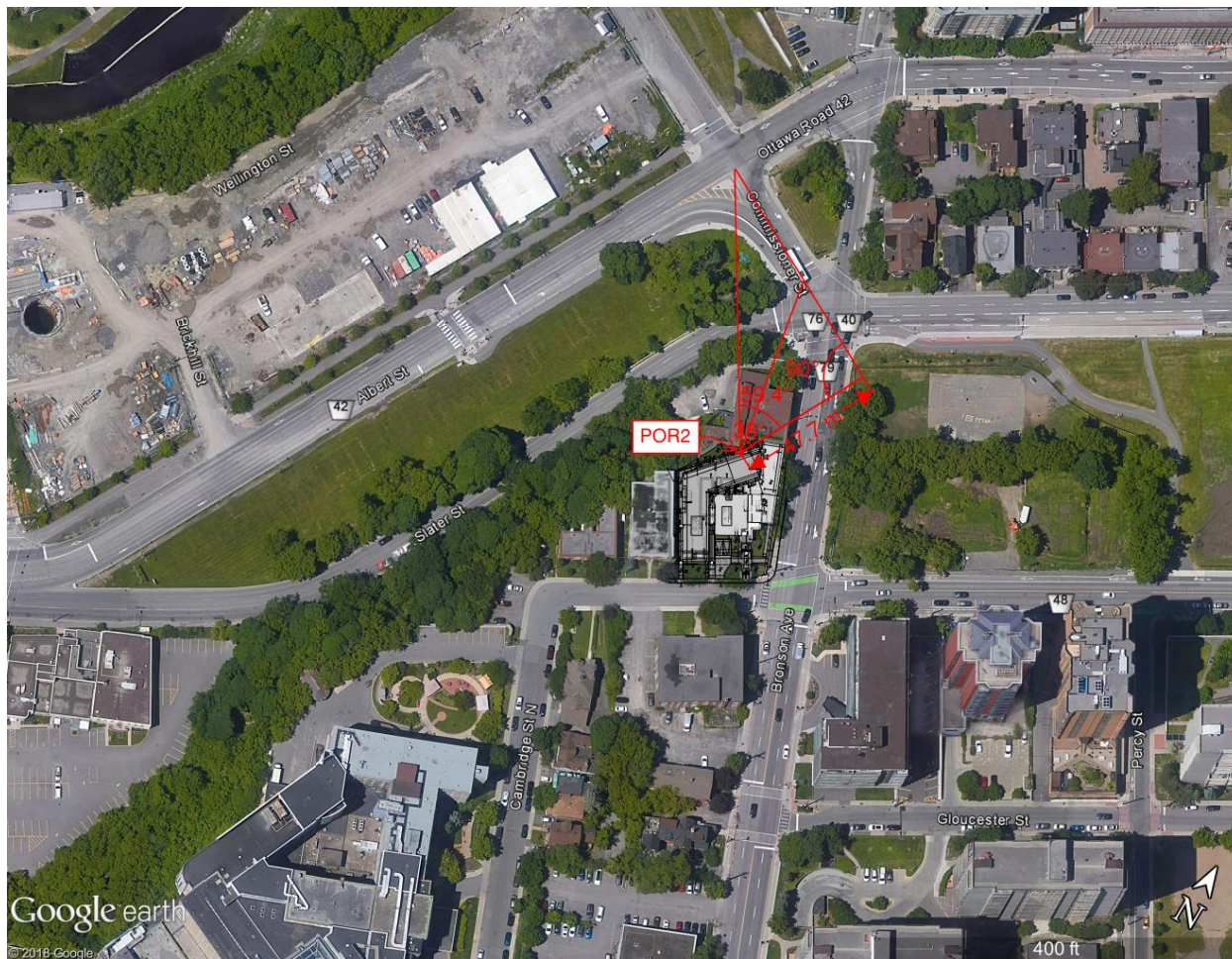
Figure 11: Distances and angles used in STAMSON 5.04 for POR2 (3 of 3)
