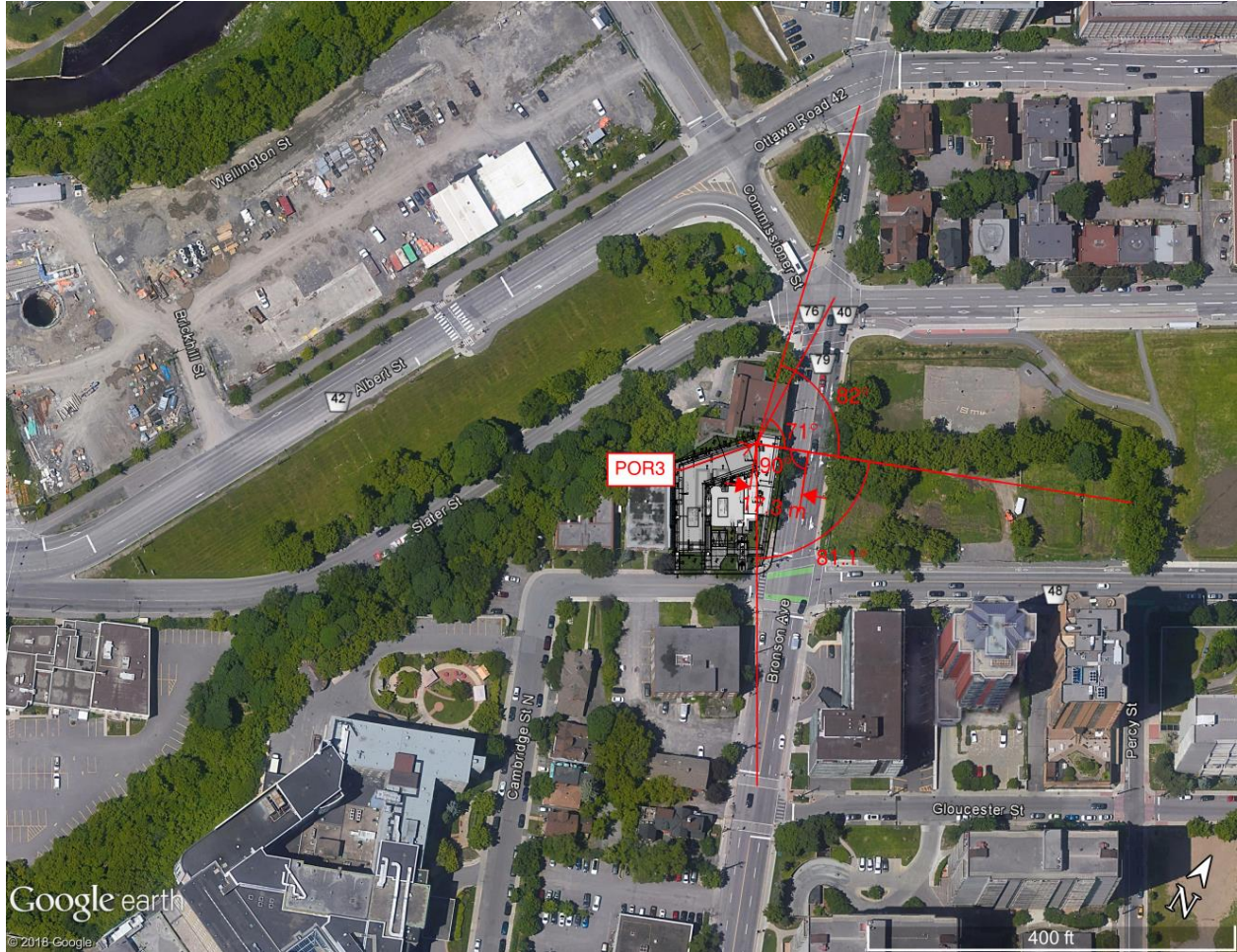
Figure 13: Distances and angles used in STAMSON 5.04 for POR3 (2 of 3)
