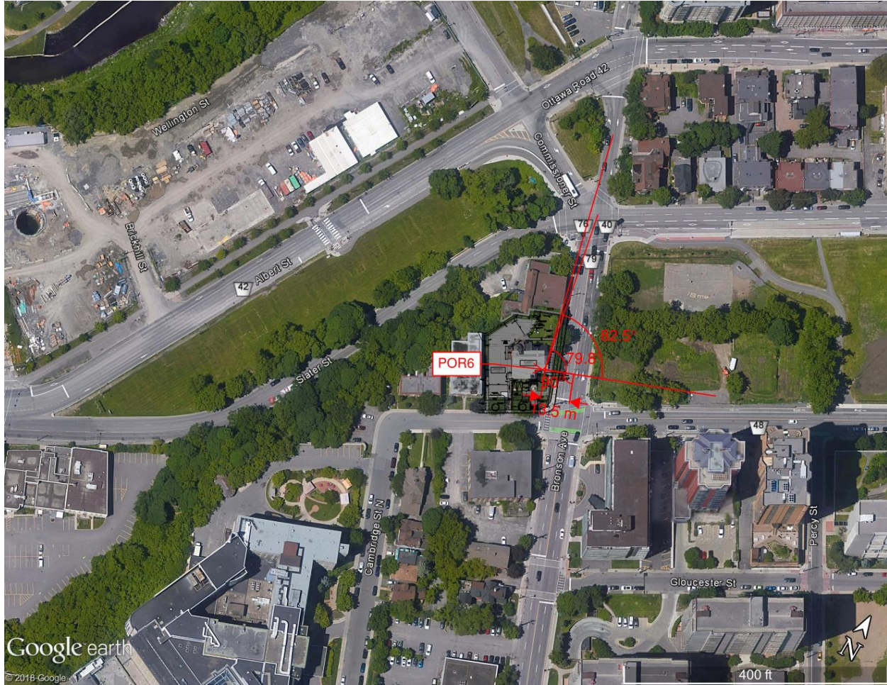
Figure 19: Distances and angles used in STAMSON 5.04 for POR6 (2 of 2)
