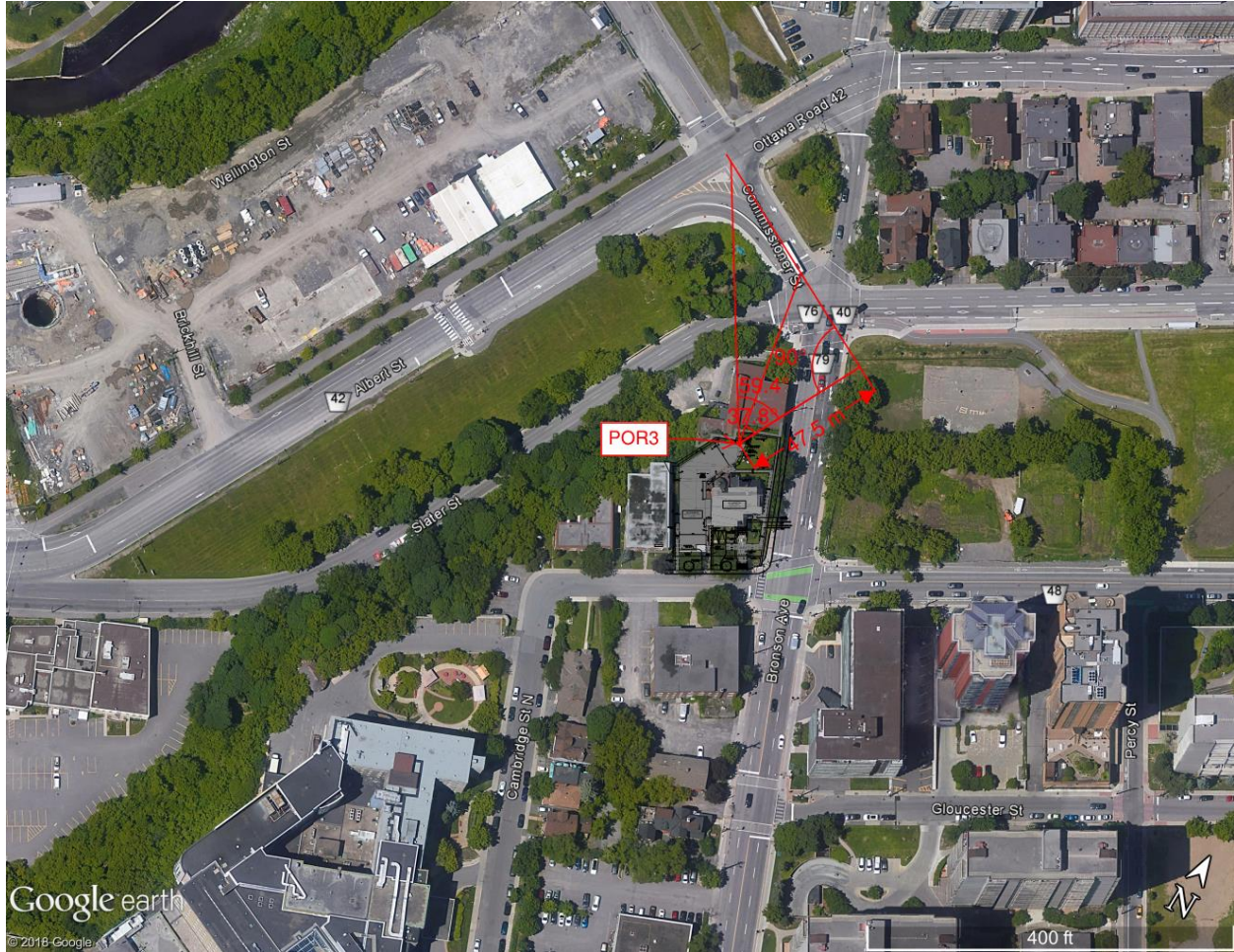
Figure 12: Distances and angles used in STAMSON 5.04 for POR3 (3 of 3)
