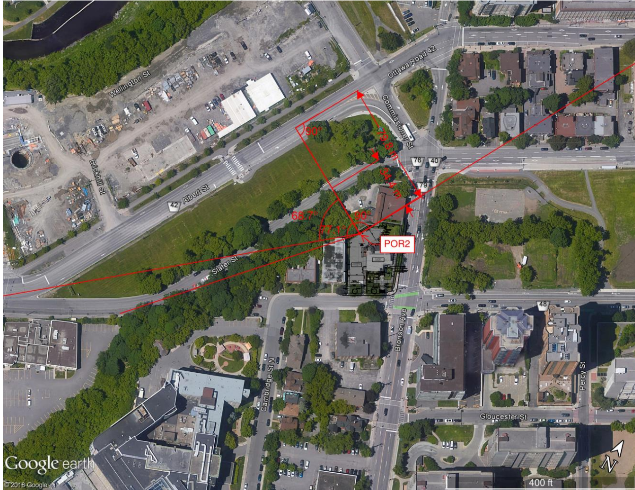
Figure 7: Distances and angles used in STAMSON 5.04 for POR2 (1 of 3)
