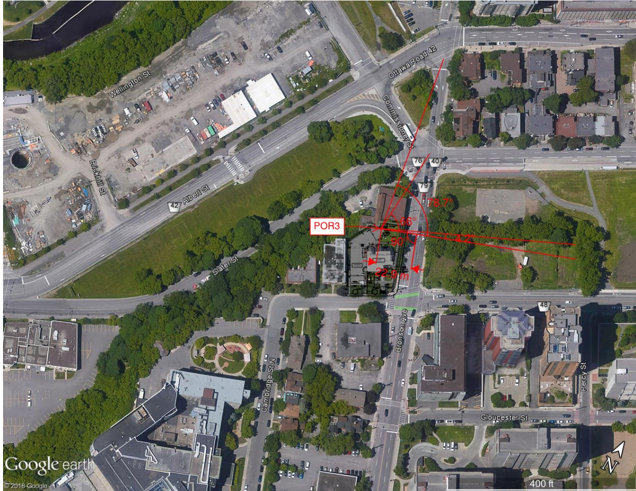
Figure 11: Distances and angles used in STAMSON 5.04 for POR3 (2 of 3)
