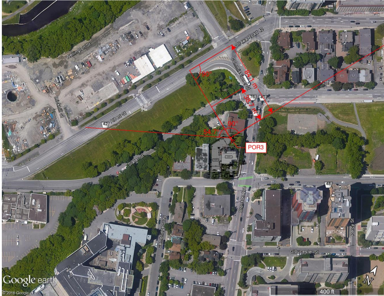
Figure 10: Distances and angles used in STAMSON 5.04 for POR3 (1 of 3)
