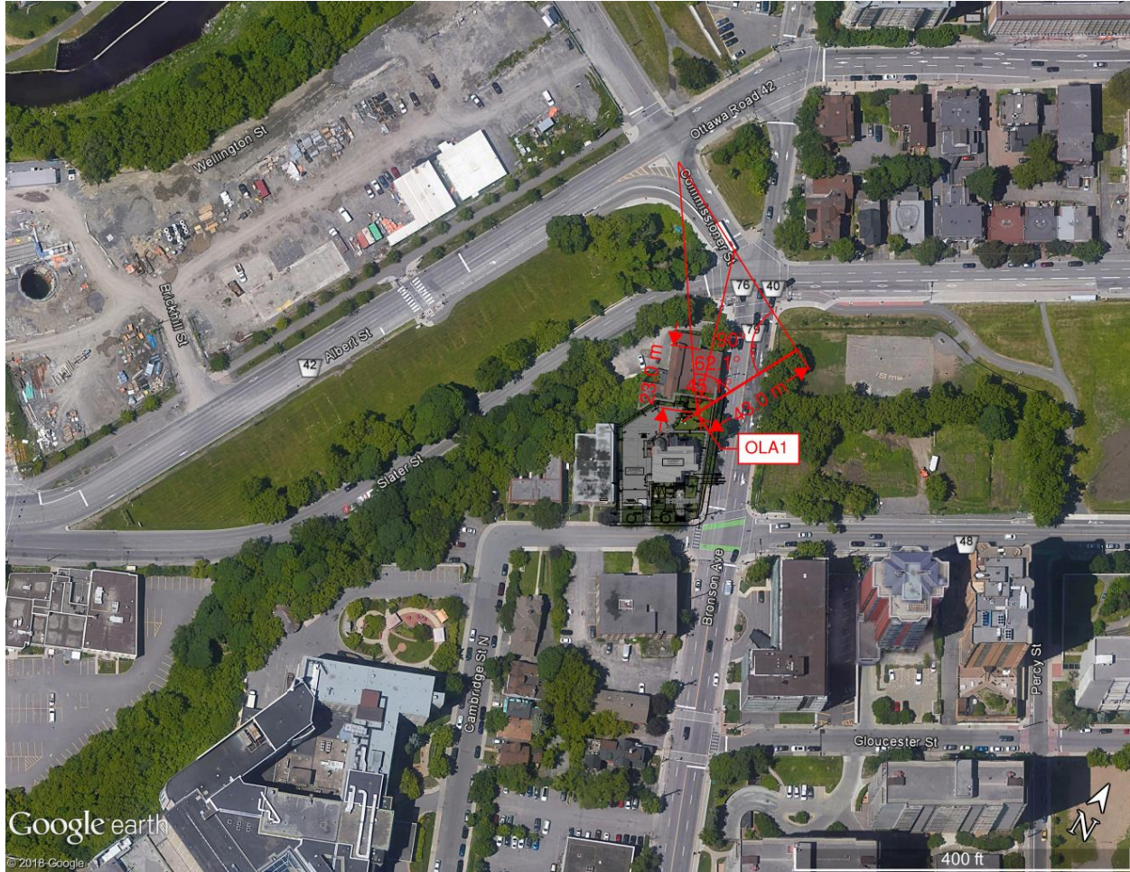
Figure 22: Distances and angles used in STAMSON 5.04 for OLA1 (3 of 3)
