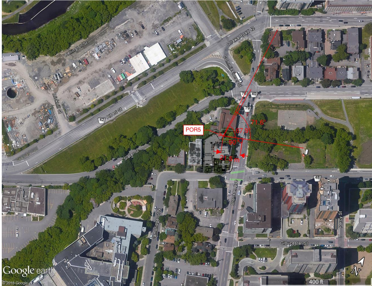
Figure 17: Distances and angles used in STAMSON 5.04 for POR5 (2 of 2)
