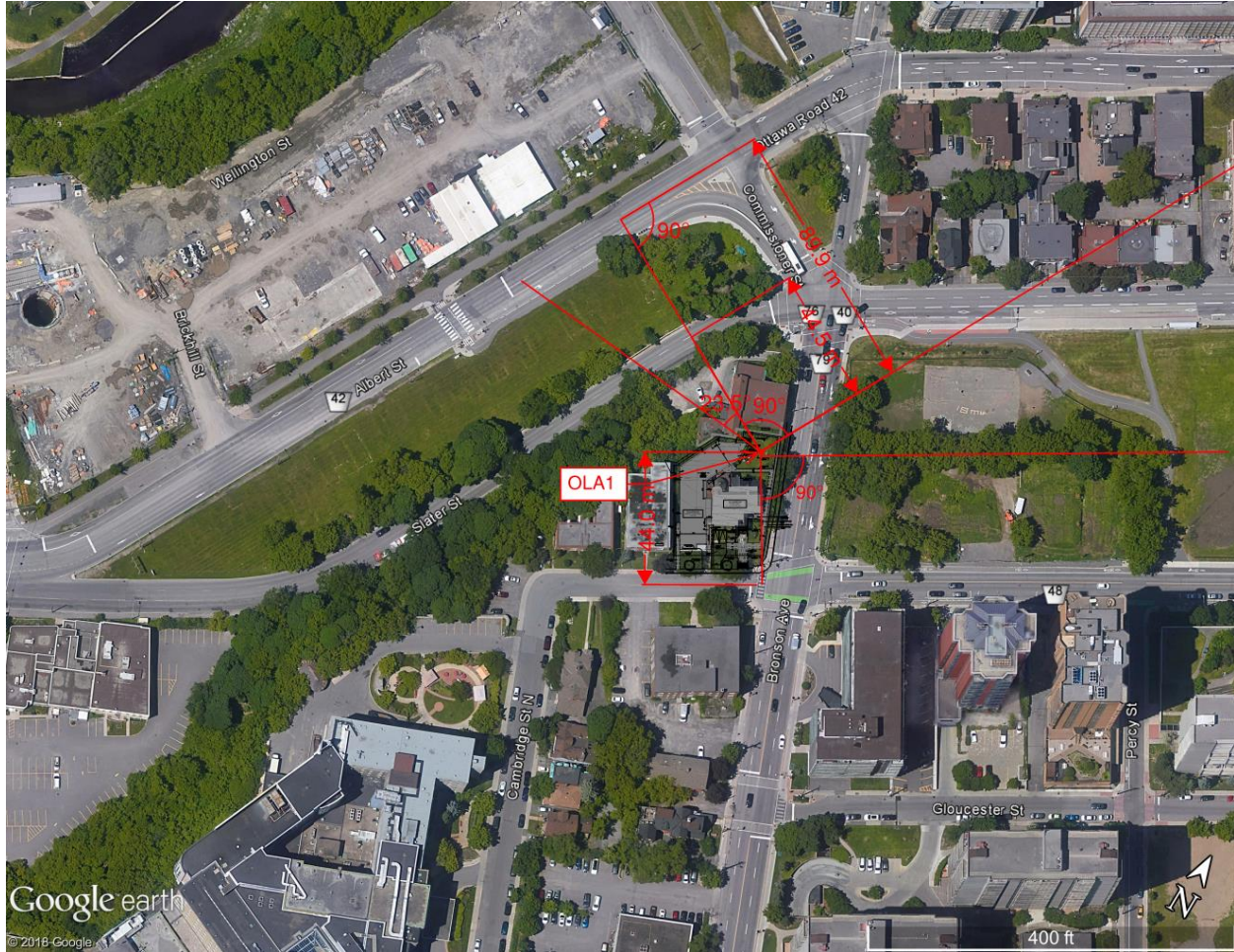
Figure 20: Distances and angles used in STAMSON 5.04 for OLA1 (1 of 3)
