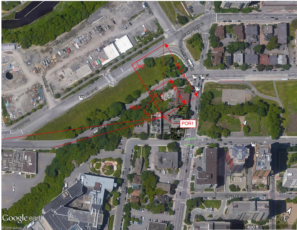
Figure 6: Distances and angles used in STAMSON 5.04 for POR1 (1 of 1)
