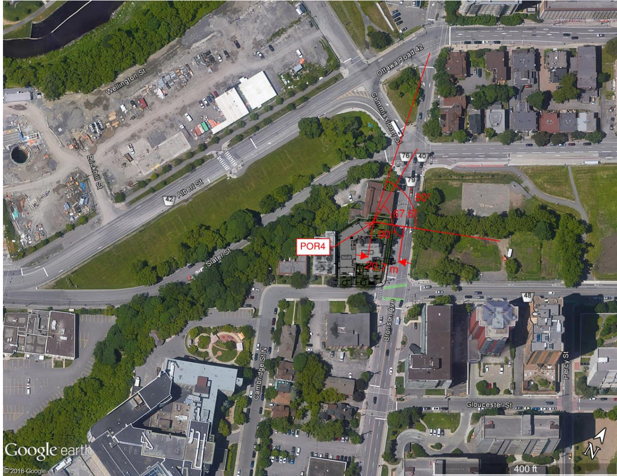
Figure 14: Distances and angles used in STAMSON 5.04 for POR4 (2 of 3)
