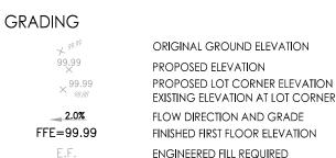
FINISHED FIRST FLOOR ELEVATION ENGINEERED FILL REQUIRED TERRACING 3:1 SLOPE MAXIMUM (UNLESS OTHERWISE SHOWN) \_ · · · · \_ · · · \_ · · · \_ PROPOSED SWALE DIRECTION OF OVERLAND FLOW PROPOSED VALVE BOX PROPOSED VALVE CHAMBER PROPOSED FIRE HYDRANT
