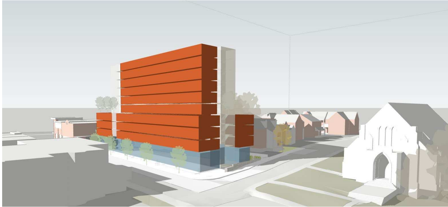
BUILDING FRONT LINE 2M SETBACK FROM PROPERTY LINE, SETBACK ABOVE 4TH STOREY TOTAL FLOORS: 10 (1 COMMERCIAL GROUND FLOOR / 3 RESIDENTIAL PODIUM FLOORS / 6 TOWER FLOORS)
