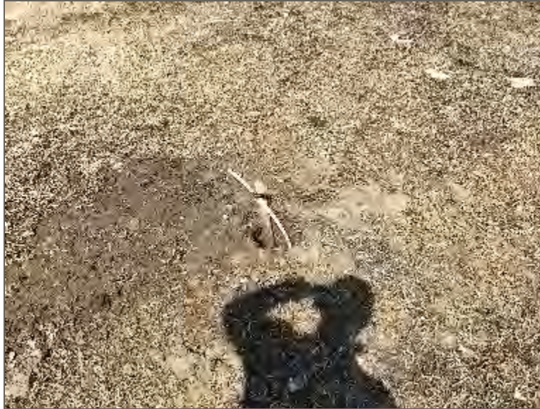
Photo 7 – Typical borehole area with associated Waterra tubing (for geotechnical purposes).
