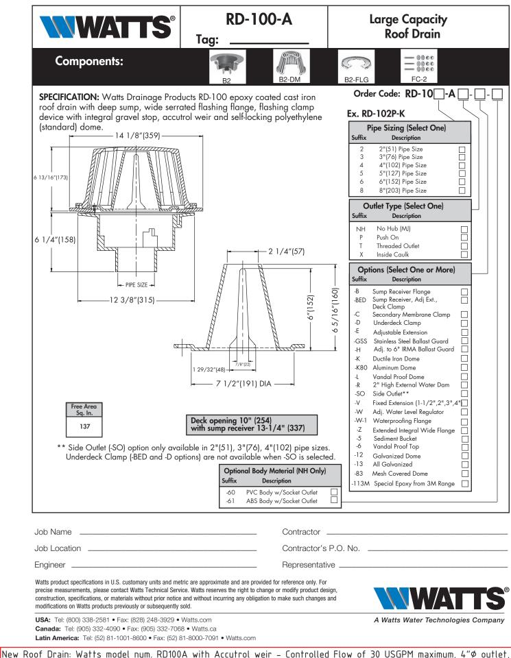
New Roof Drain: Watts model num. RD100A with Accutrol weir – Controlled Flow of 30 USGPM maximum, 4"Ø outlet, equipped with adjustable flow control up to 6" of head, epoxy-coated cast-iron construction with weirs, under deck clamp, gravel guard and sump.
