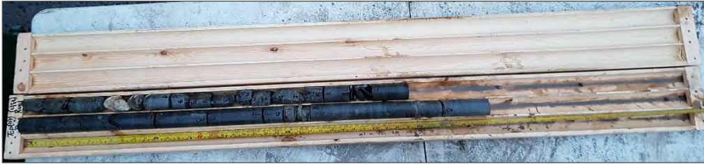
Photo 1 – Borehole BH4, Rock Core (Runs 1 and 2)
