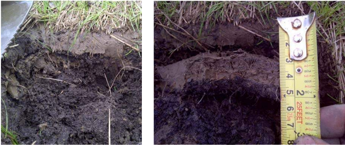
Figure 5.0 – Field Verification of Topsoil Depths using Common Garden Spade (Aquafor Beech, 2011)
