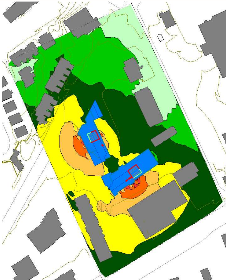
FIGURE 5: HVAC NOISE CONTOURS DAYTIME (37.4 M ABOVE GRADE, WITH 4-M NOISE SCREEN AND ACOUSTIC LOUVRE)
