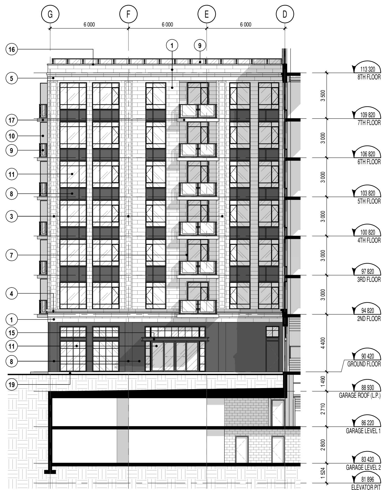
NORTH ELEVATION (PARTIAL) 1: 150
