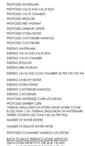
150mm SANITARY SERVICE PVC SDR 28 @ 1% MIN 19mm PEX TUBING WATER SERVICE C/W CURB STOP AND SERVICE POST VILLAGE TOWN HOME SERVICES (NO BASEMENTS) 0mm STORM SERVICE PVC SDR 28 @ 1% MIN
