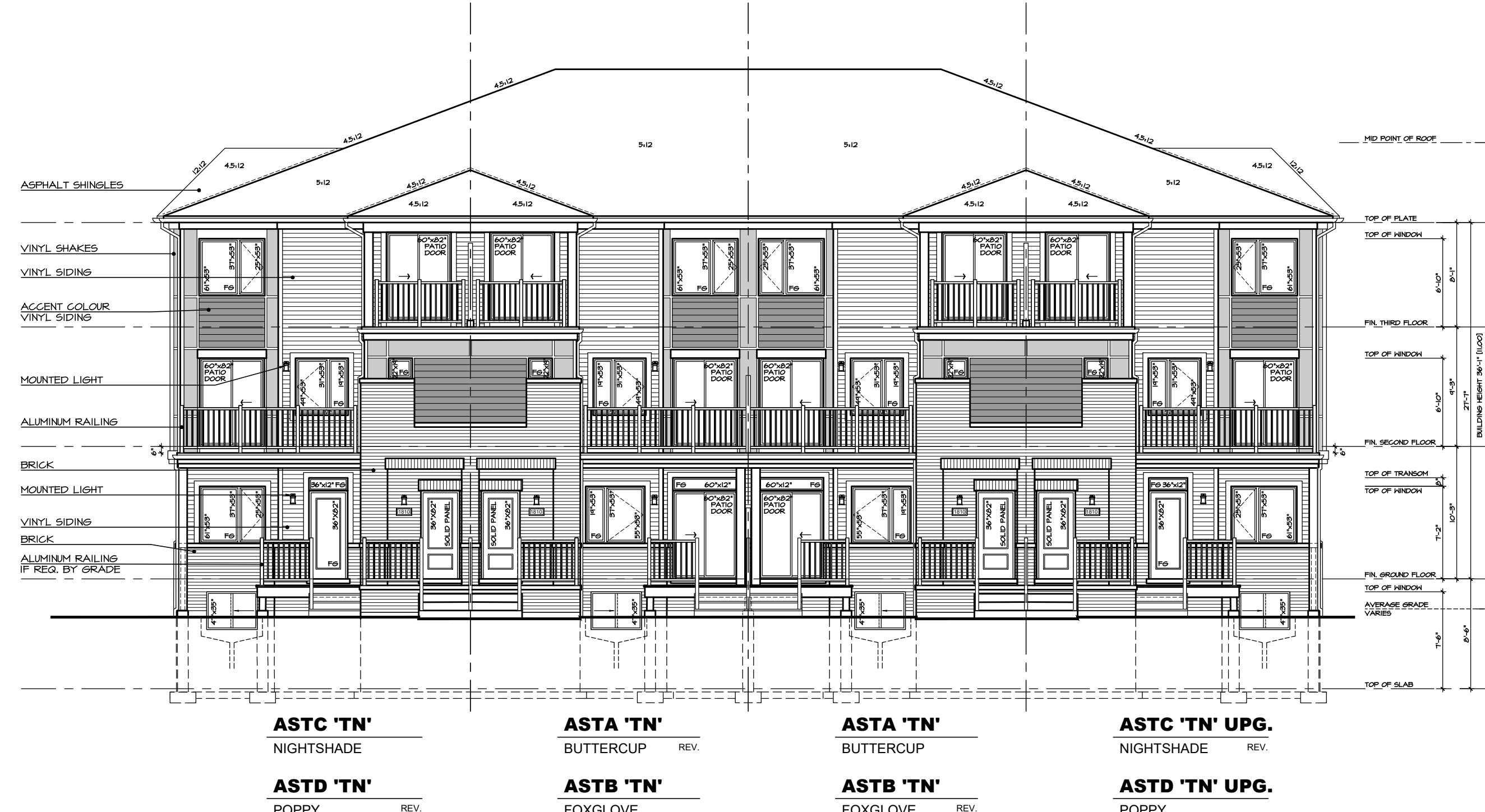
REAR ELEVATION - STREET SIDE
