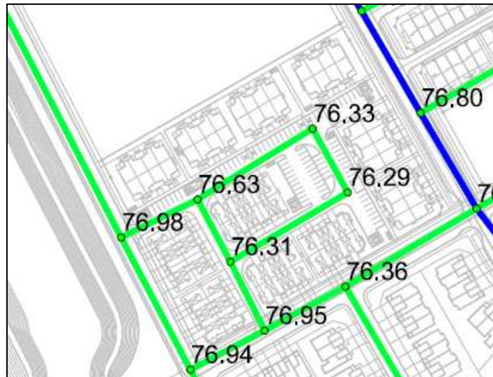
Figure 3.4: Post SUC Zone Reconfiguration - Ultimate Condition PKHR Pressure Results (psi)
