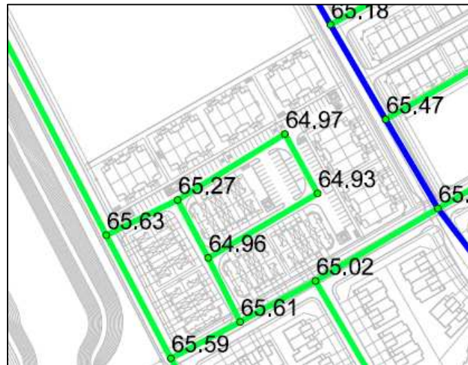
Figure 3.2: Existing Zone - Ultimate Condition PKHR Pressure Results (psi)
