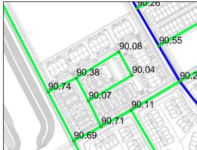
Figure 3.2: Existing Zone - Ultimate Condition PKHR Pressure Results (psi)
