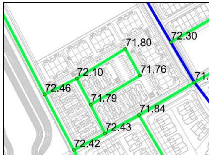
Figure 3.4: Post SUC Zone Reconfiguration - Ultimate Condition PKHR Pressure Results (psi)
