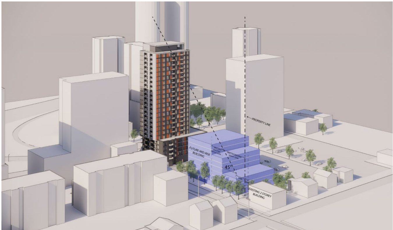
Figure 7: Illustration of Transition from Proposed Building to Low-rise Neighbourhood, using 45-degree Angular Plane.
