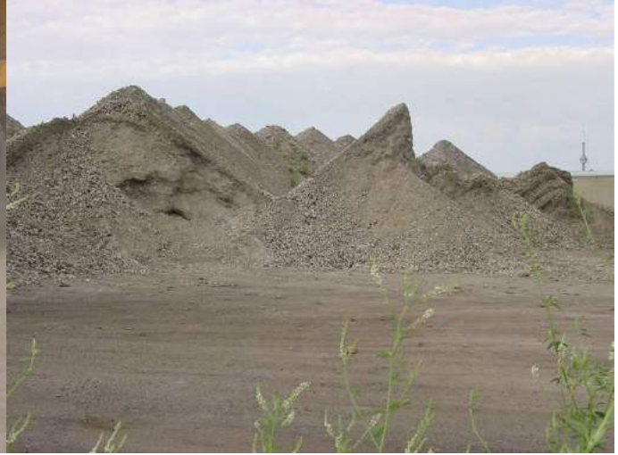
Figure 16. Unprotected Storage Piles
