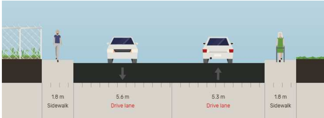
Figure 4-4. Commissioner Street - Existing Cross-Section
