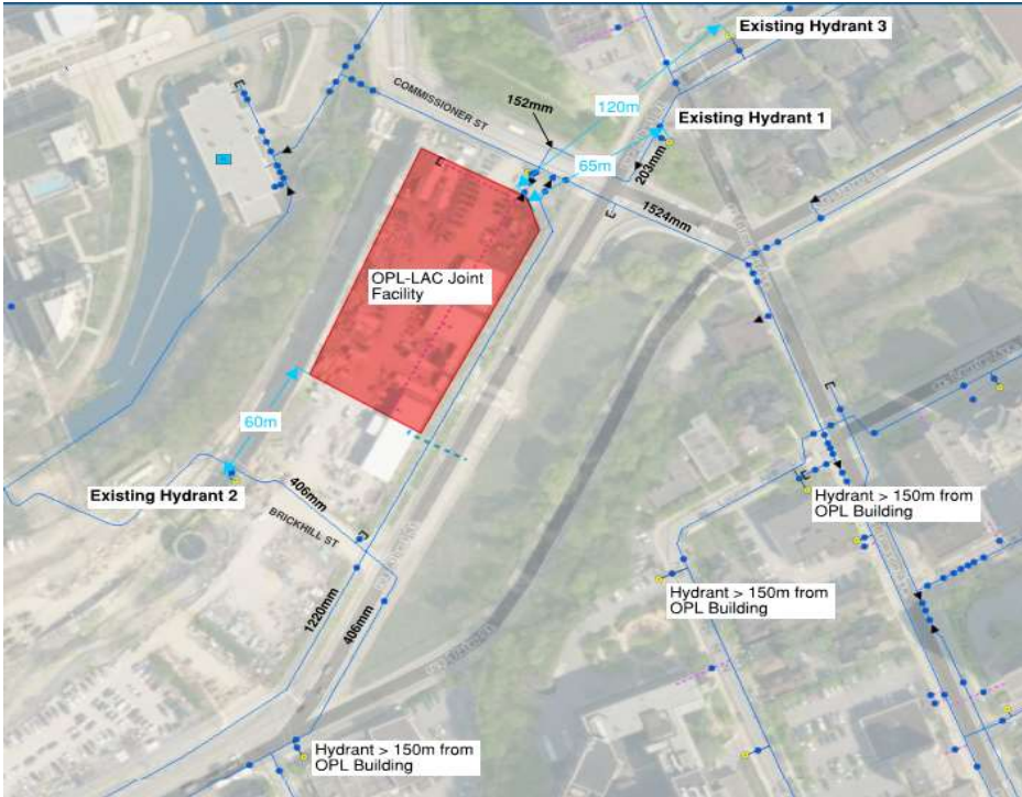
Figure 1: Adjacent Buildings & distances to hydrants
