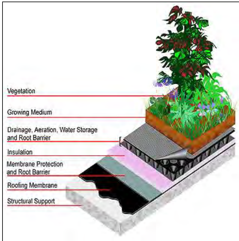
Figure 4.2.5 Green roof layers
