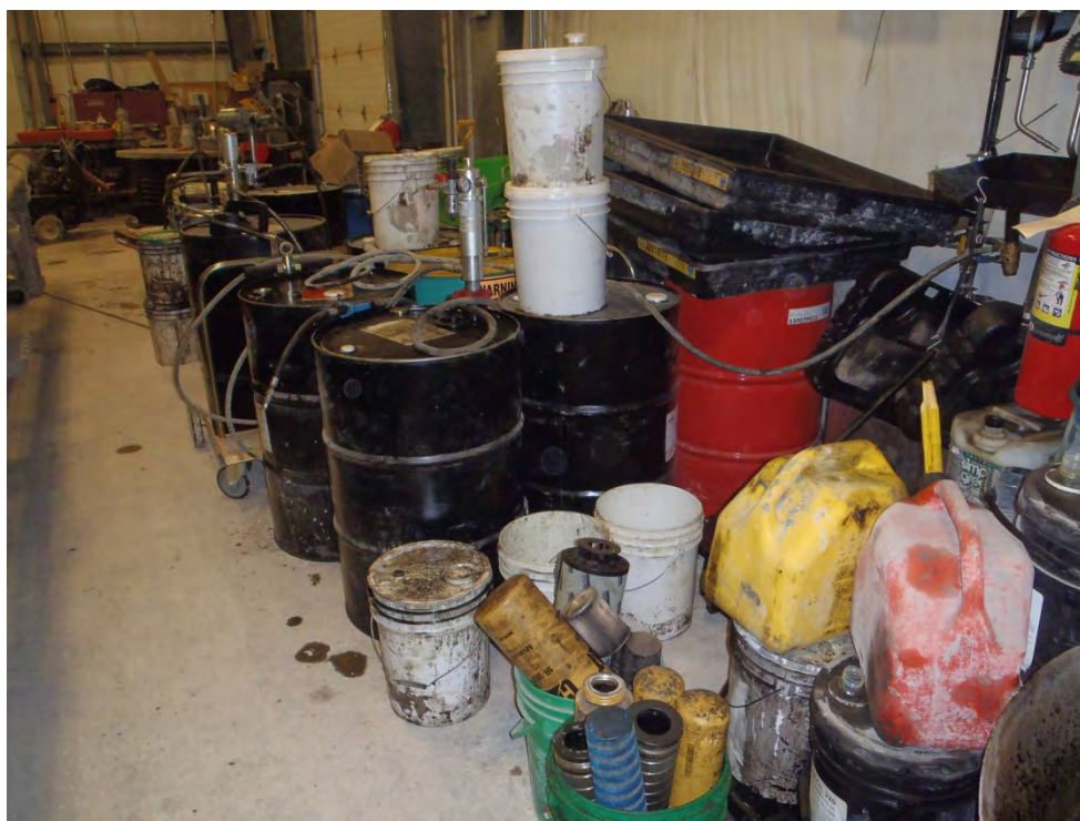
Photograph 24: Minor drip stains noted on concrete. Containers not stored in secondary containment. Containers include hydraulic oil, gear oil, motor oil, transmission oil, etc.
