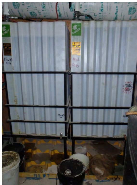
Photograph 30: Bulk storage (870 L containers) of 15w40 CJ4 engine oil and Hyd. 46 (hydraulic oil).
