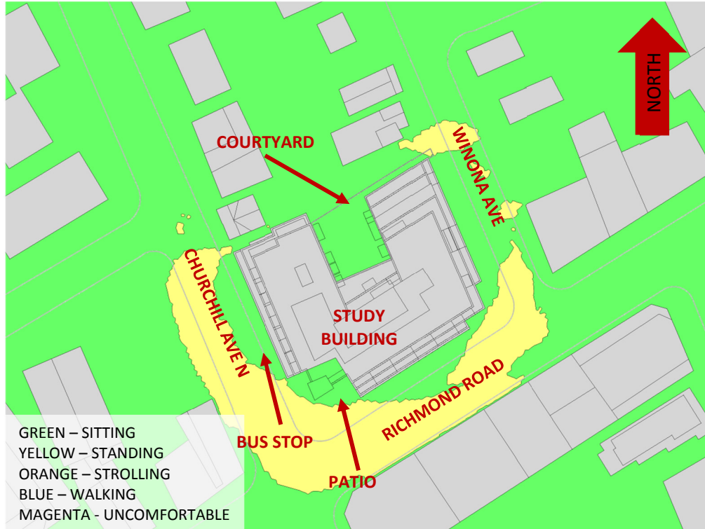
FIGURE 3A: SPRING – WIND CONDITIONS AT GRADE LEVEL
