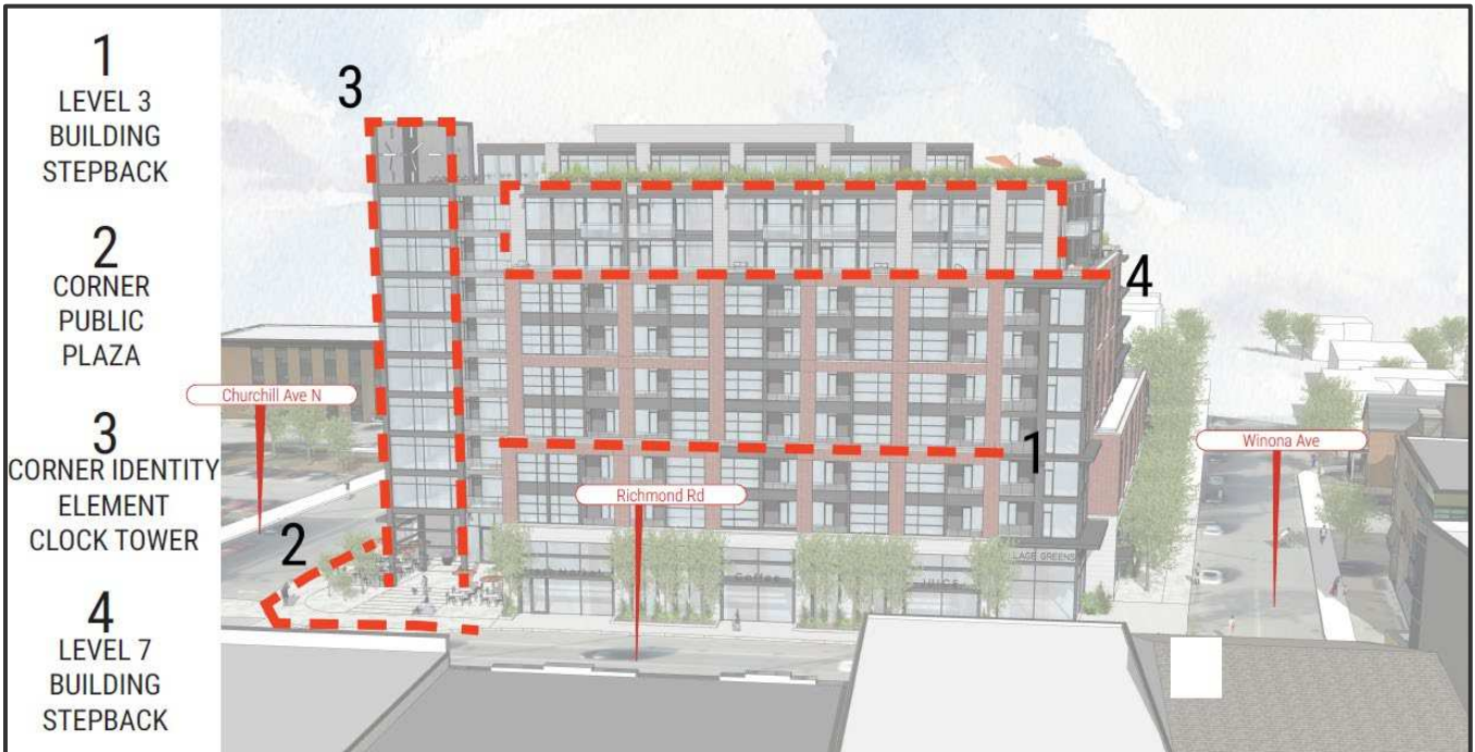
Figure 10: South Elevation along Richmond Road, showing the building form and features
