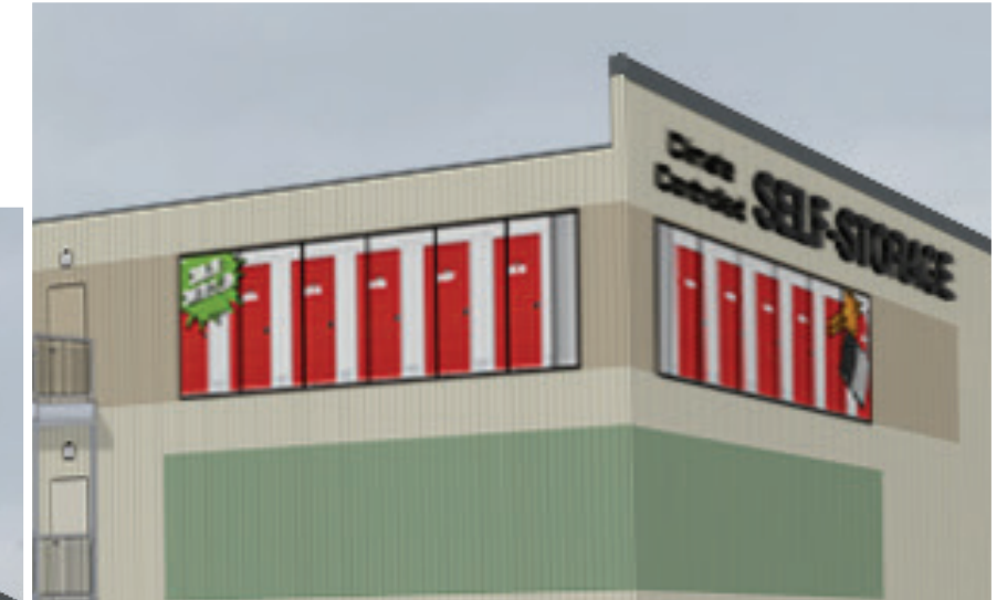
FAUX WINDOW DECALS ON ALUMINUM TO PROVIDE FENESTRATION & RETAIL APPEARANCE
