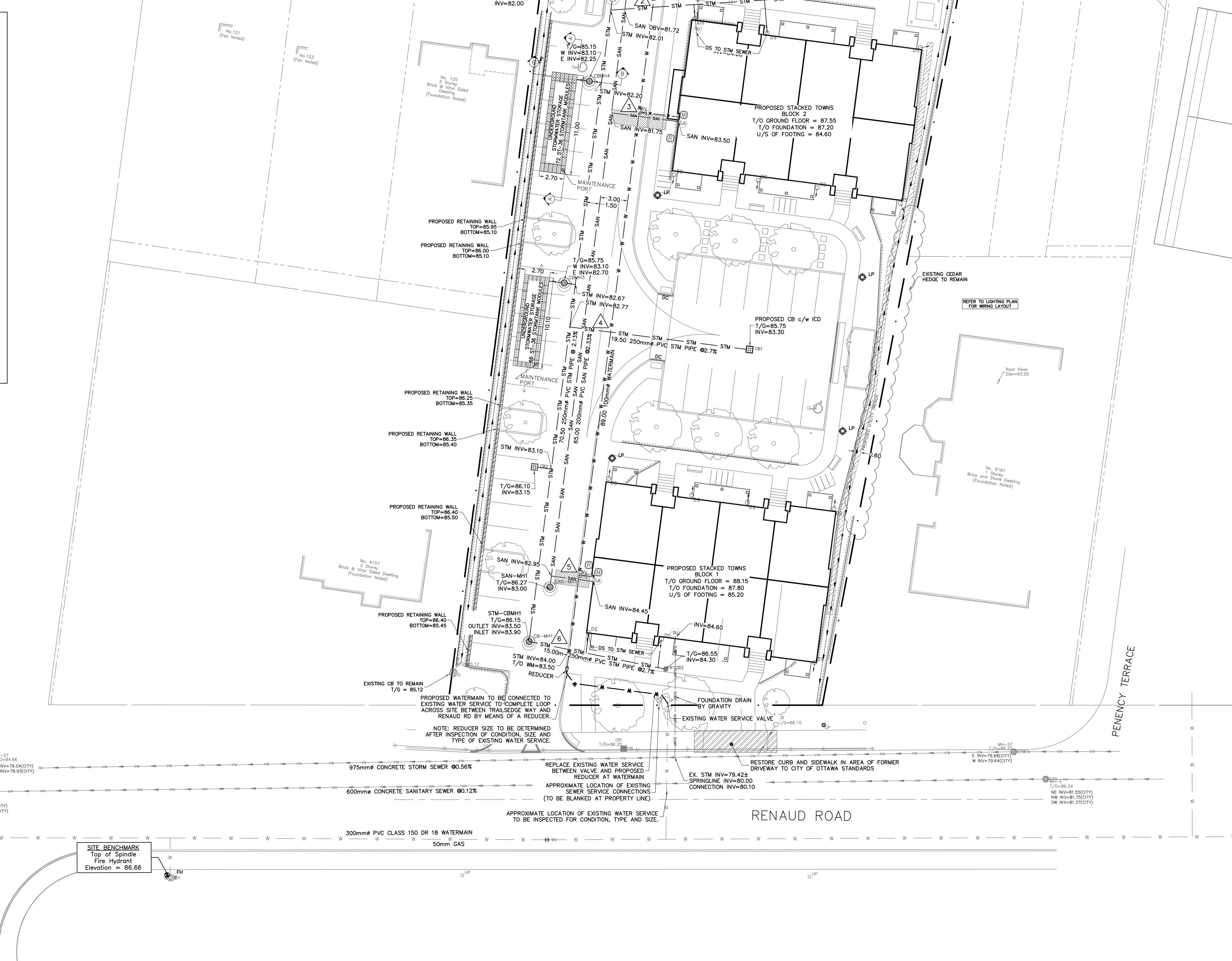
SITE SERVICING PLAN SCALE = 1:250
