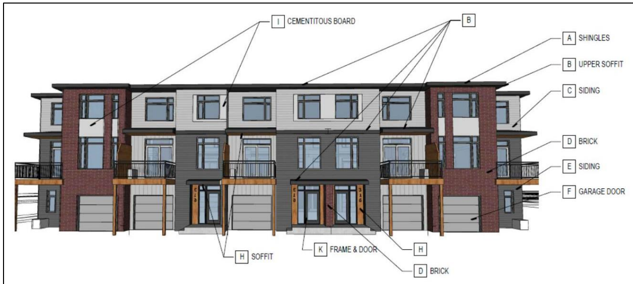
Figure 5: Conceptual townhouse colour and materials selection sheet prepared by Rosaline J. Hill Architect Inc., dated February 2019.
