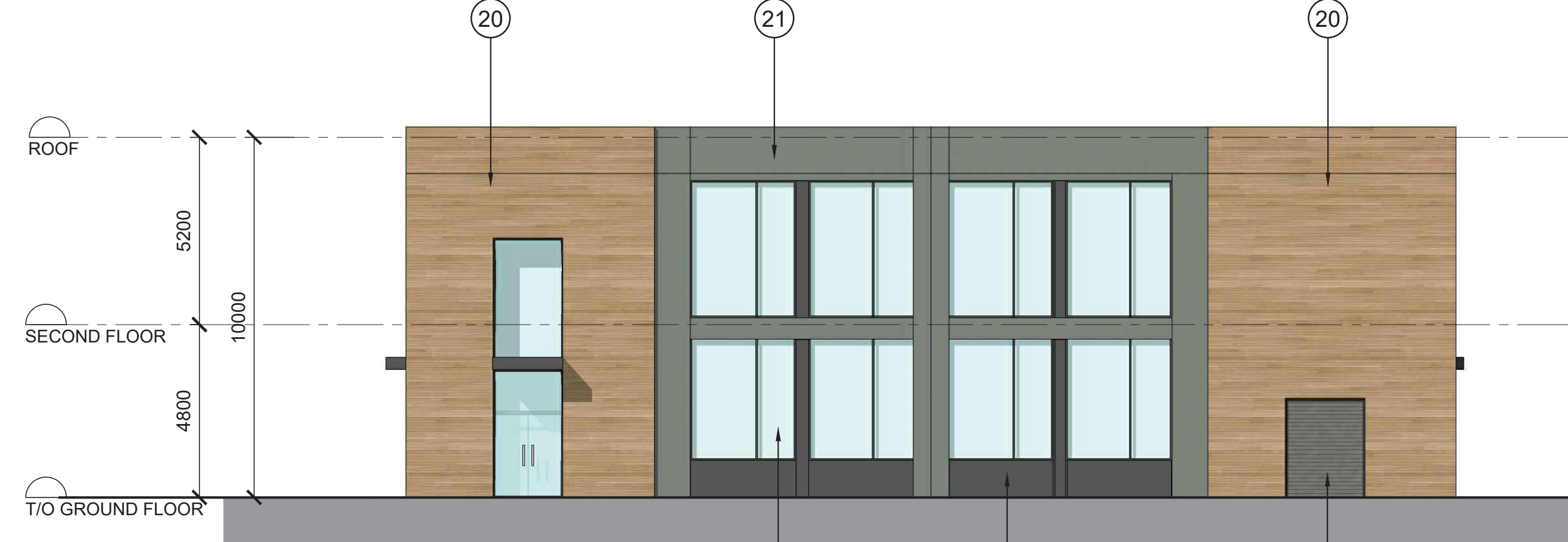
7 EAST ELEVATION SCALE = 1:125 A-01
