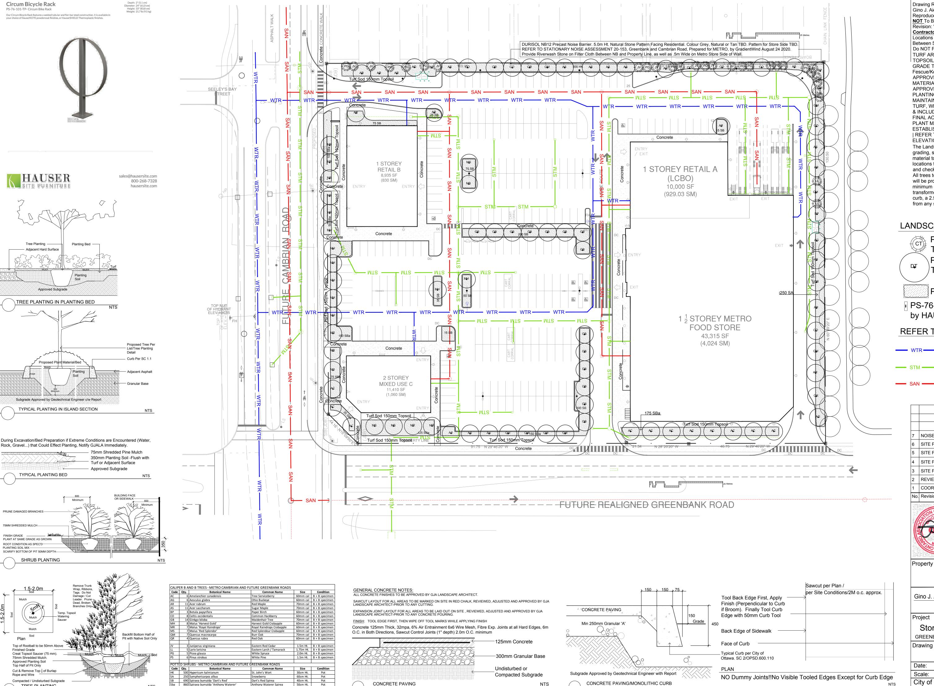
32 MPA C2 c/w FLOAT FINISH - TOOL EDGE FIRST, THEN WIPE OFF TOOL MARKS WHILE APPLYING FINISH
