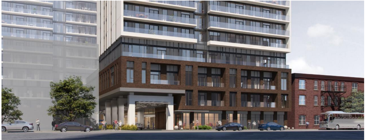
Figure 24: The 2-storey entrance highlighted in the lighter material helps to ground the north tower and creates a comfortable through-block link. The commercial style glazing at the ground floor references Bank Street retail; the use of unit masonry and a traditional colour palette support the Bank Street character by introducing a finer grain rhythm to the street frontage. Source: Graziani & Corazza Architects 2021.
