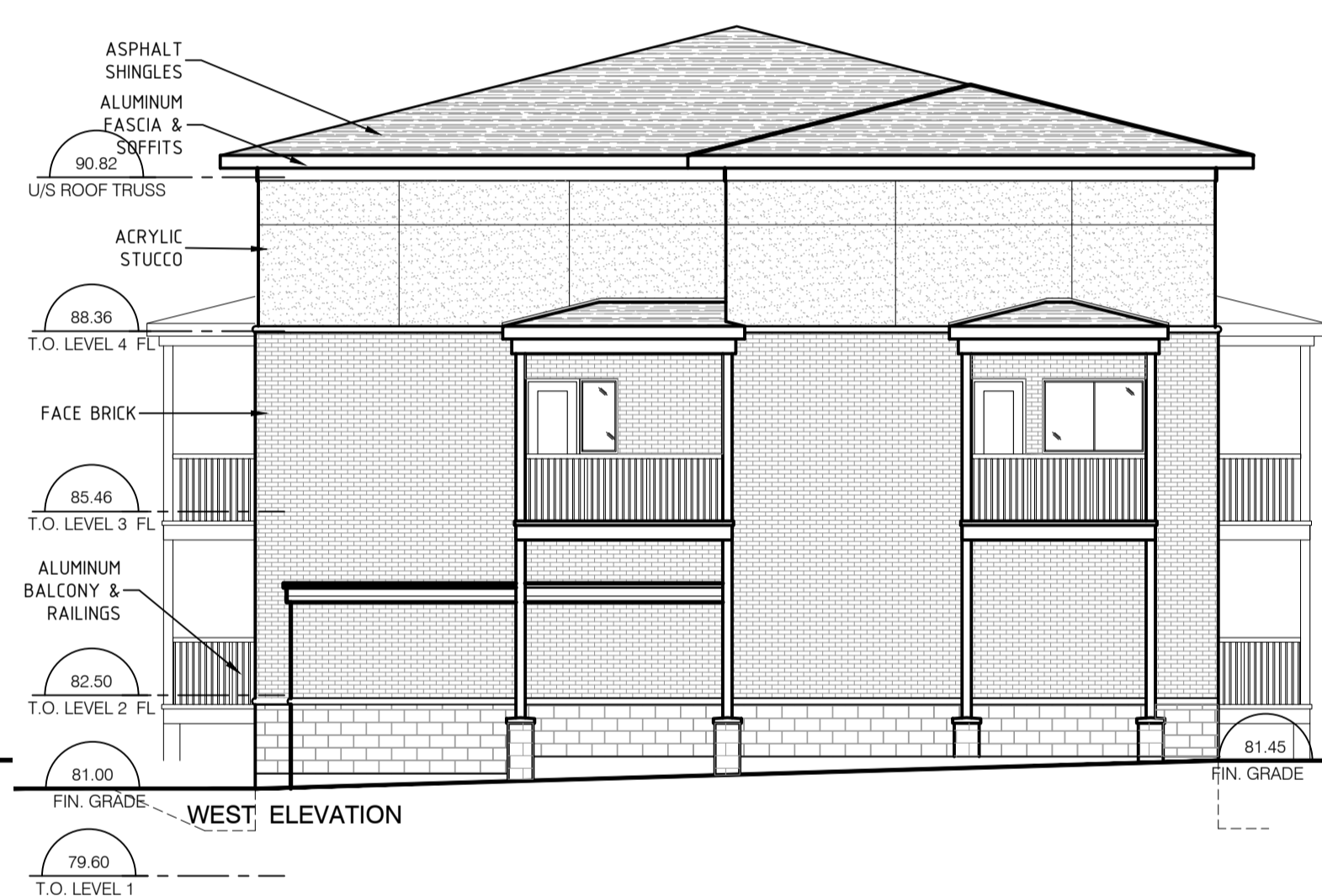
4 TOWNHOUSE BUILDING - WEST ELEVATION A100 SCALE : 1:100
