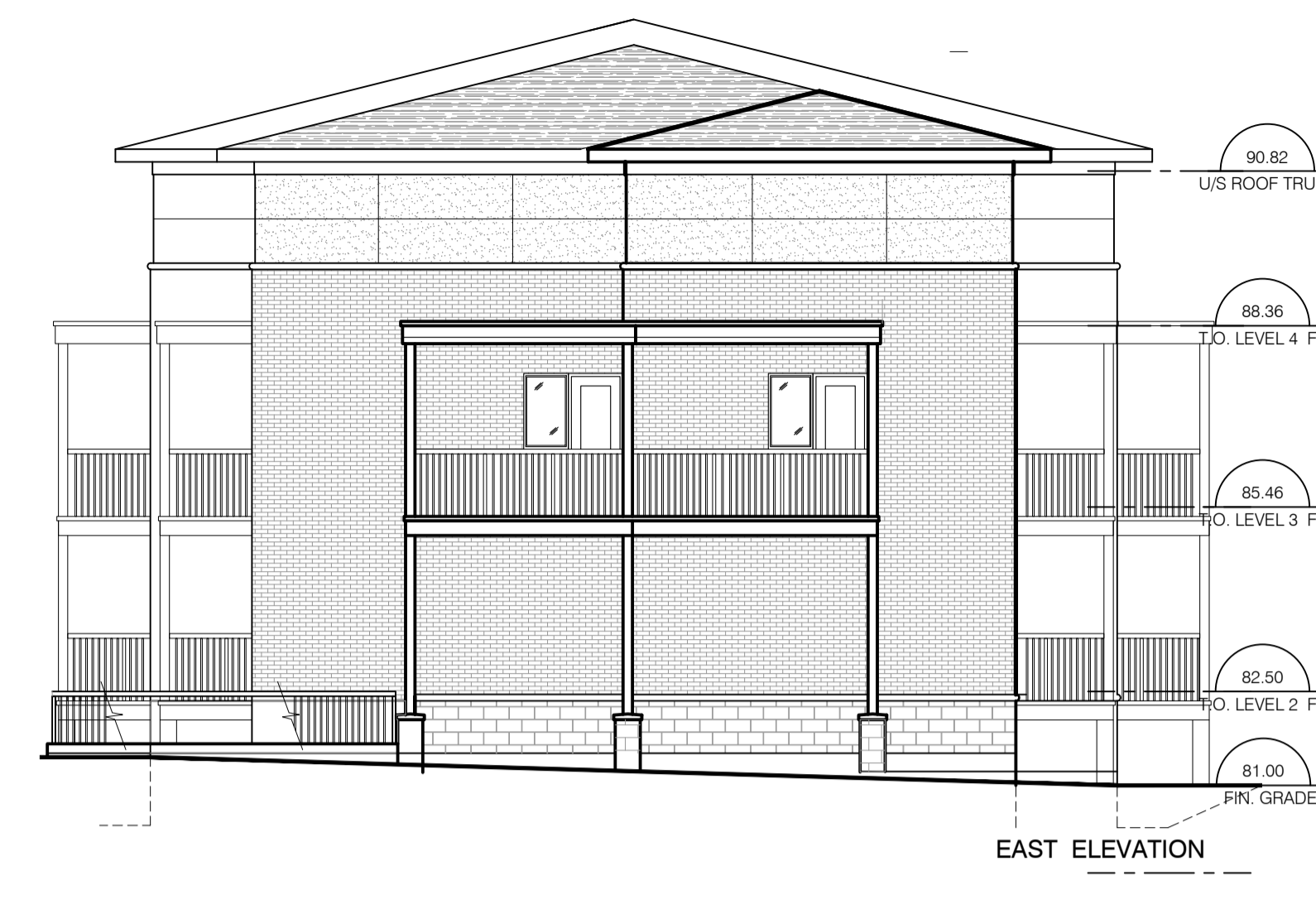
2 TOWNHOUSE BUILDING - EAST ELEVATION SCALE : 1:100
