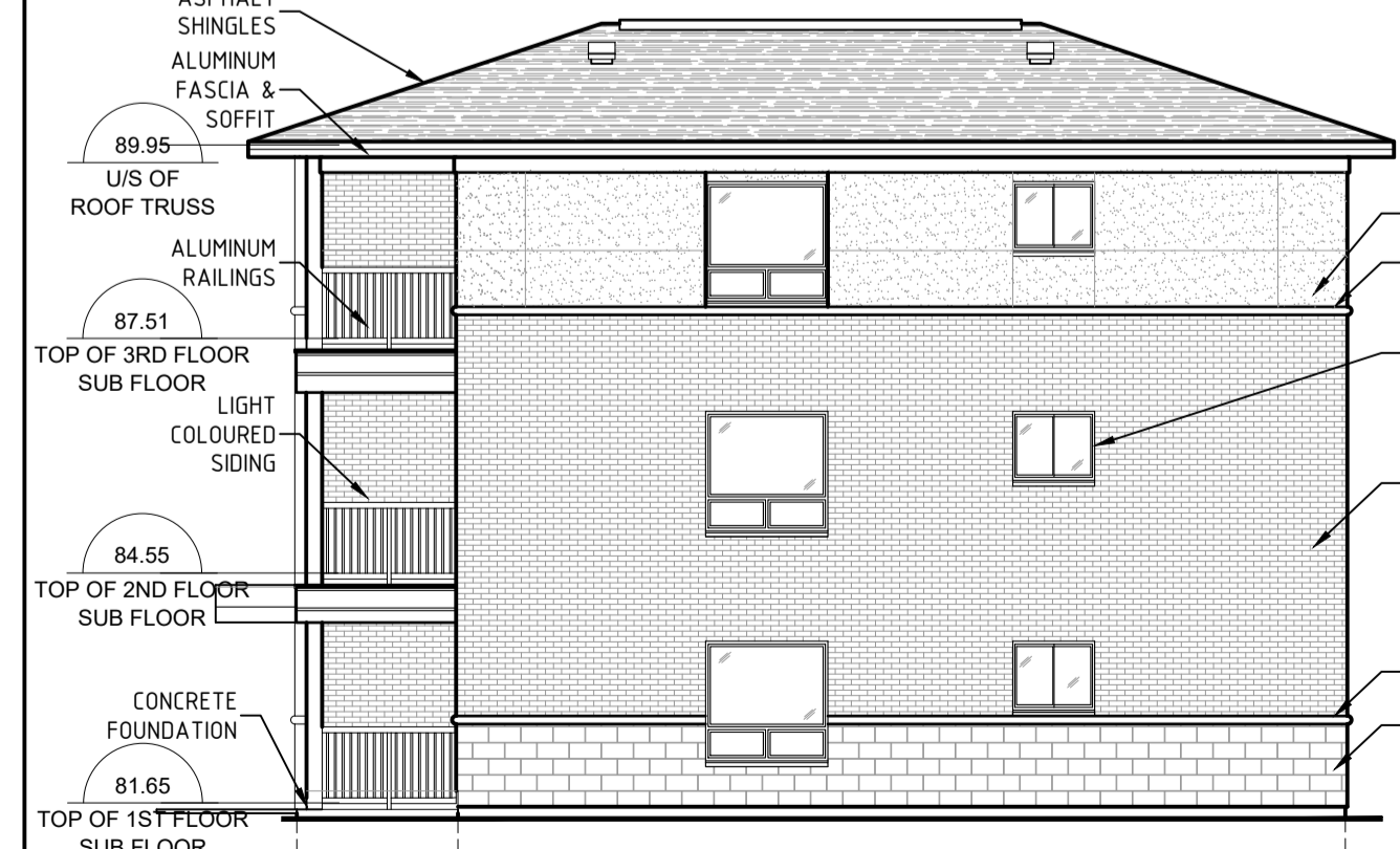
3 TRIPLEX BUILDING - SIDE ( NORTH ) ELEVATION SCALE : 1:100
