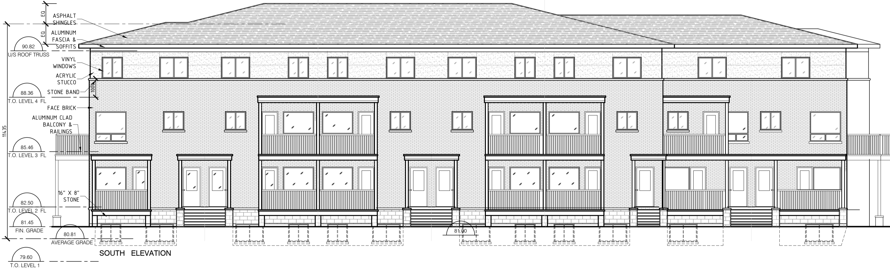
3 TOWNHOUSE BUILDING - SOUTH ELEVATION SCALE : 1:100
