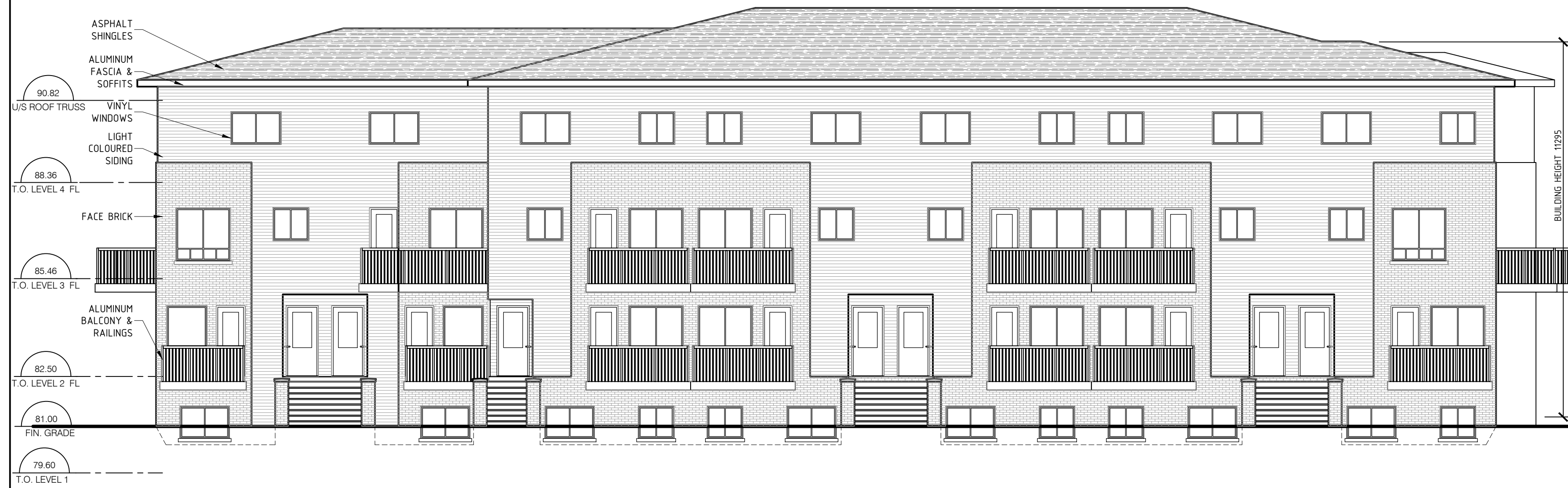
1 TOWNHOUSE BUILDING - NORTH ELEVATION SCALE : 1:100
