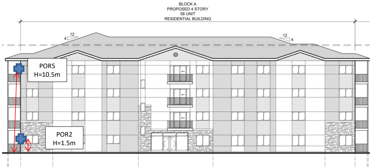
Figure 4.7 – South face elevation view showing POR2 and POR5.
