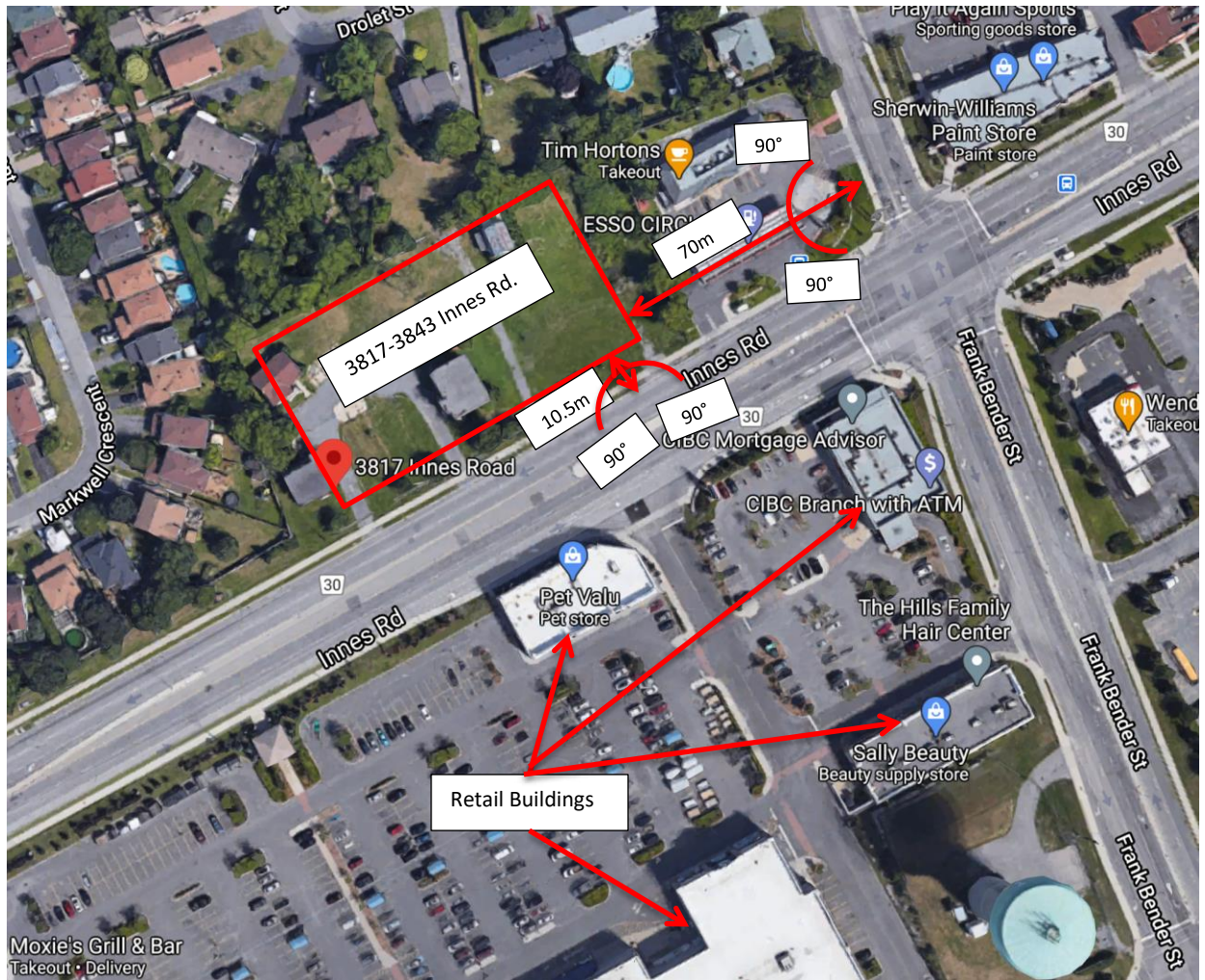
Figure 2.2 – Surrounding area 3817-3843 Innes Rd. with locations, distances and angles of relevant noise sources
