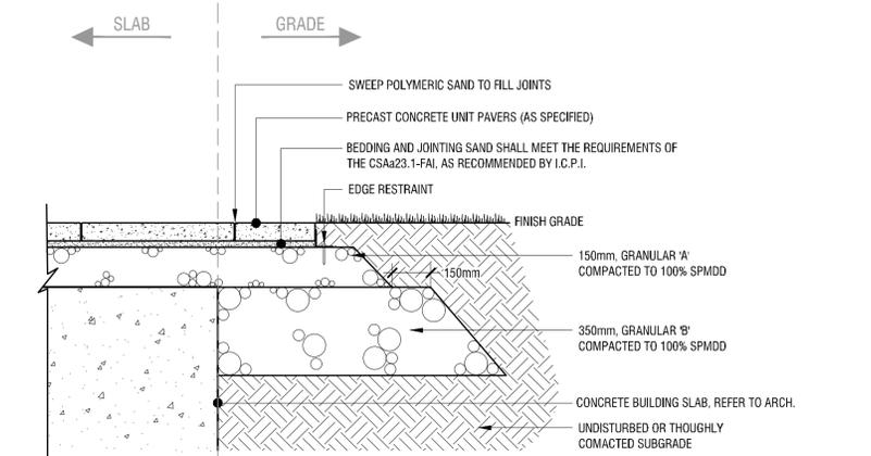
**5 HEAVY-DUTY CONCRETE UNIT PAVING AT BUILDING PODIUM**
