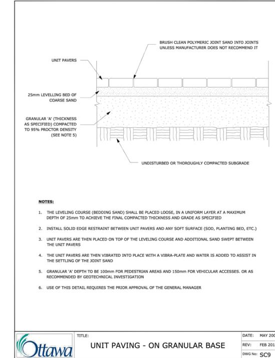
**4 STANDARD CONCRETE UNIT PAVING**
