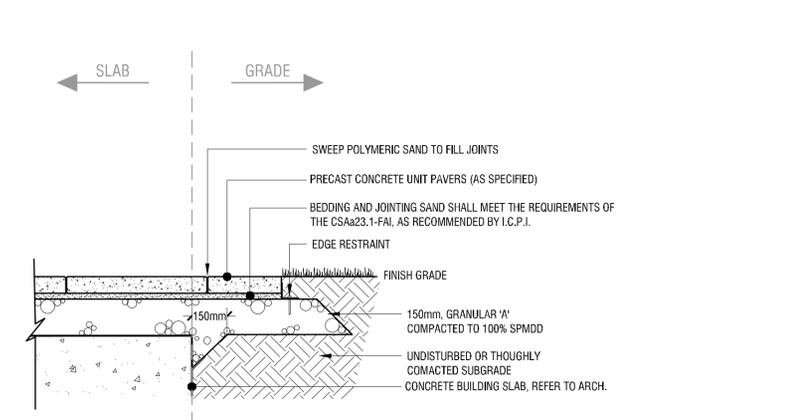
**6 LIGHT-DUTY CONCRETE UNIT PAVING AT BUILDING PODIUM**
