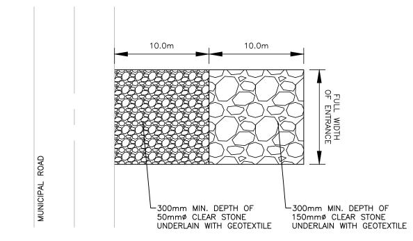
1. MUD MAT TO BE UNDERLAIN WITH A GEOTEXTILE FABRIC. 2. SEDIMENT SHALL BE CLEANED FROM MUNICIPAL RIGHT—OF—WAYS AS REQUIRED.
