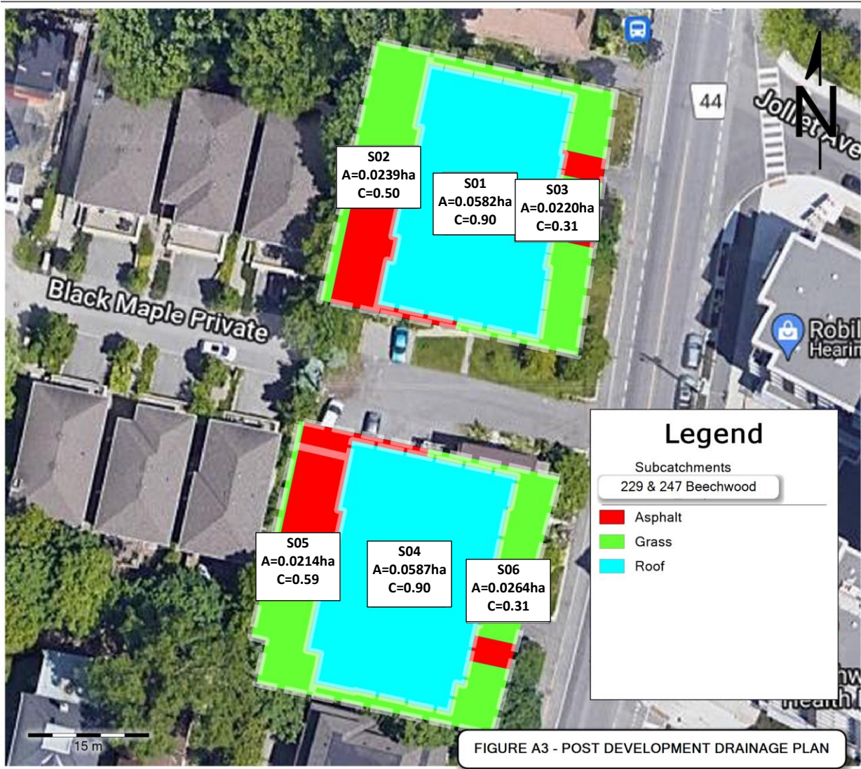
Figure 7-1 – Post-Development Storm Drainage
