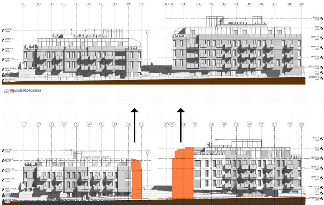
Figure 31: Elevations illustrating the reduction on massing with the revised proposal
