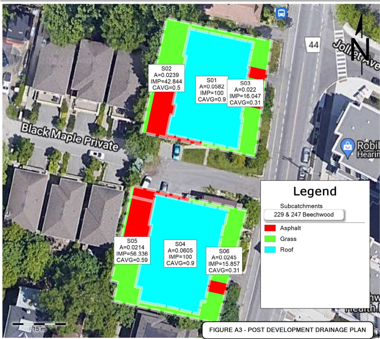
Figure 7-1 – Post-Development Storm Drainage
