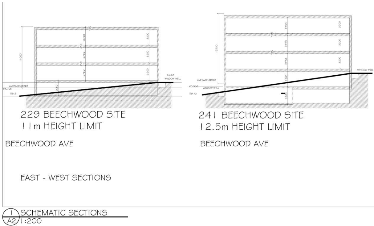
Figure 11: Schematic sections of the two buildings. The upper height limit for both buildings is 12.5m or four storeys. Source: Woodman Architects April 2020
